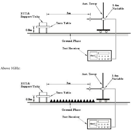
The radiated emissions were performed in the 3 meters chamber test site, using the setup accordance with the ANSI C63.4-2014. The specification used was with the FCC Part 15 B Class B limits.
