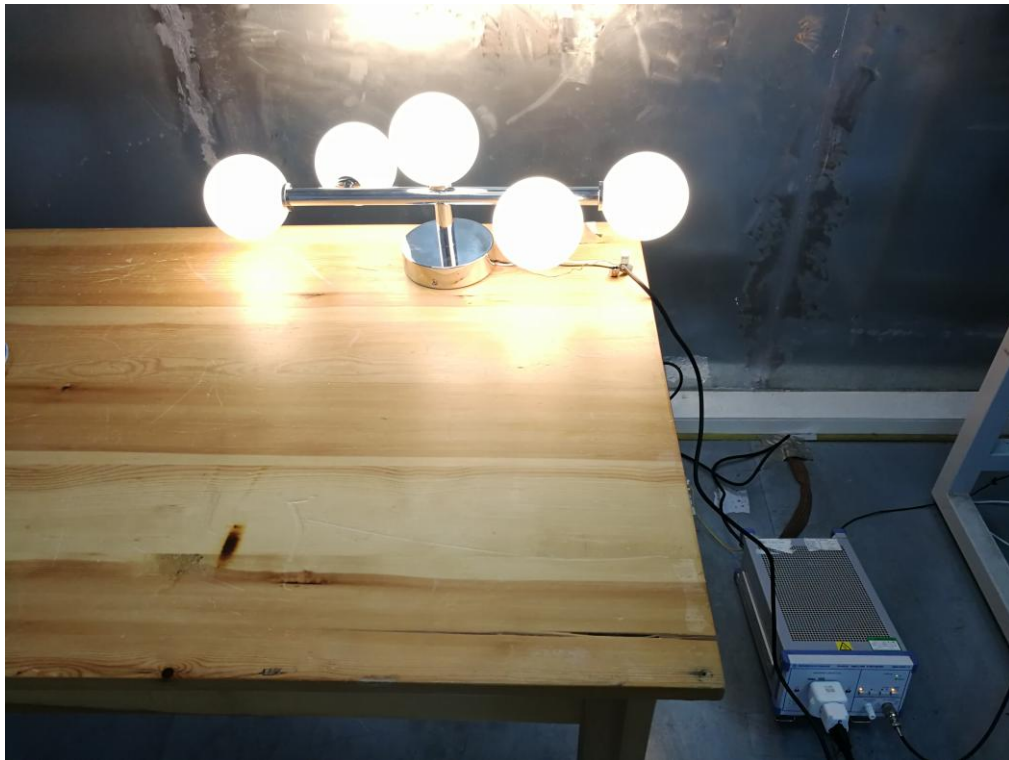
Photo of Power Line Conducted Measurement
