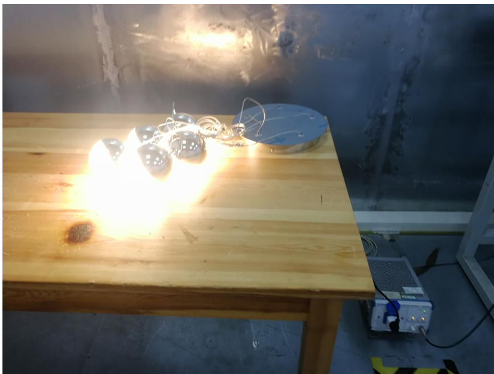
Photo of Power Line Conducted Measurement
