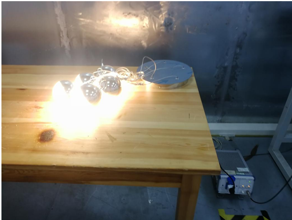
Photo of Power Line Conducted Measurement
