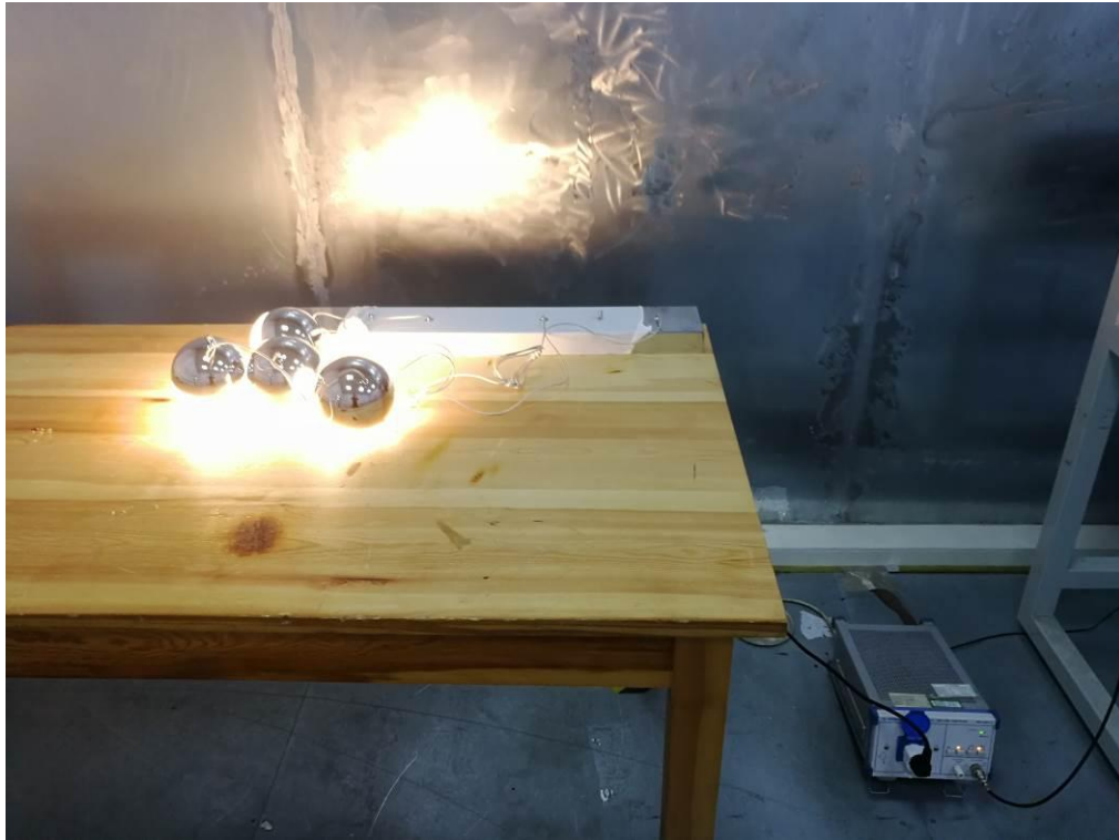
Photo of Power Line Conducted Measurement
