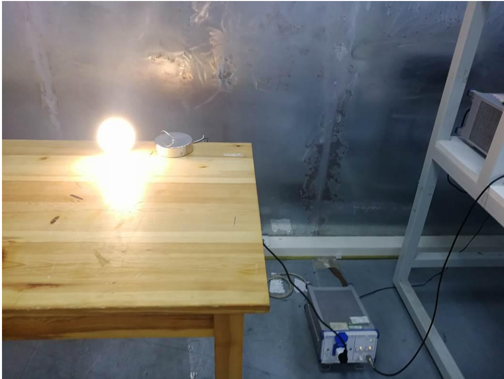
Photo of Power Line Conducted Measurement
