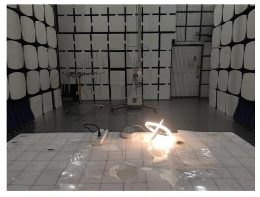
Radiated Emission below 30MHz-AC adapter charge mode
