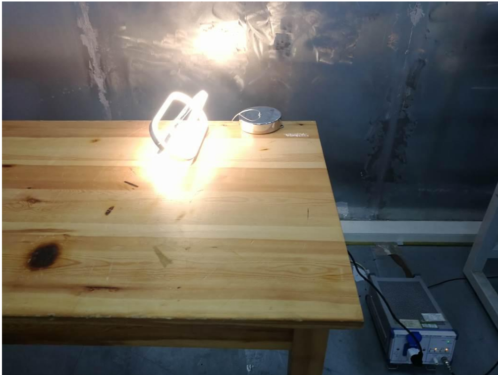
Photo of Power Line Conducted Measurement
