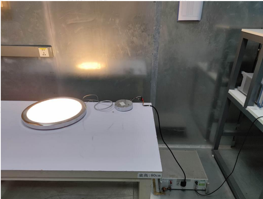
Photo of Power Line Conducted Measurement
