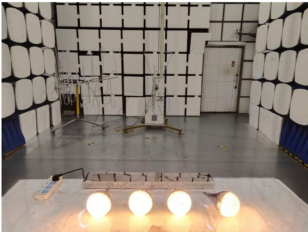
Photo of Radiated Measurement
