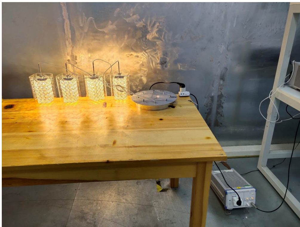
Photo of Power Line Conducted Measurement
