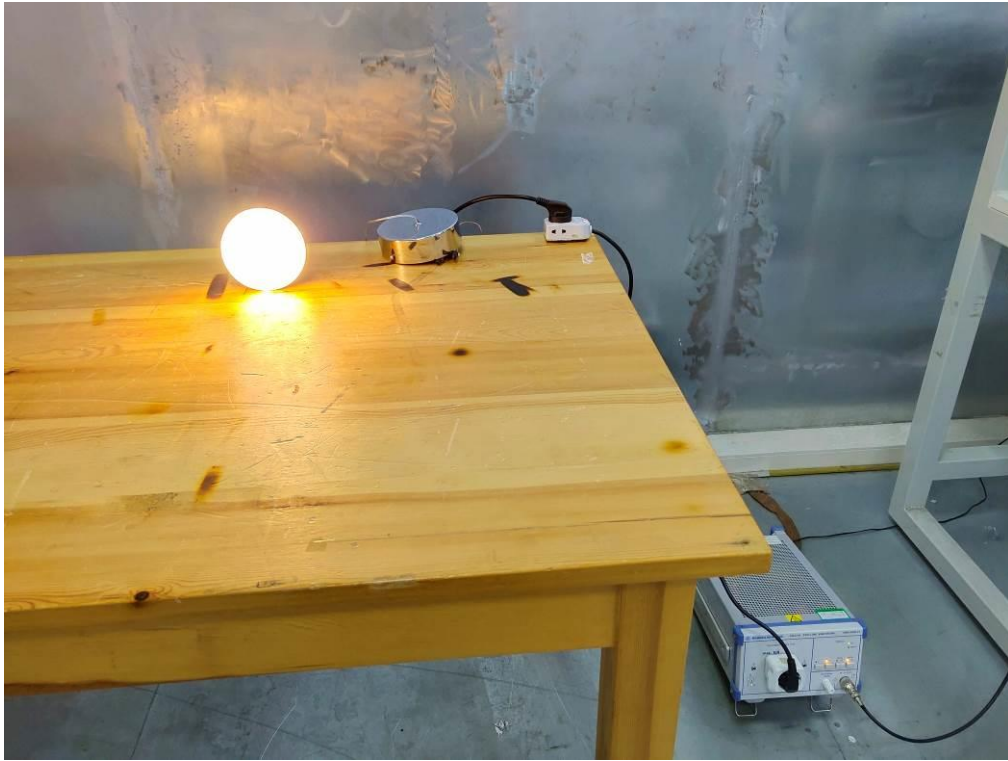
Photo of Power Line Conducted Measurement
