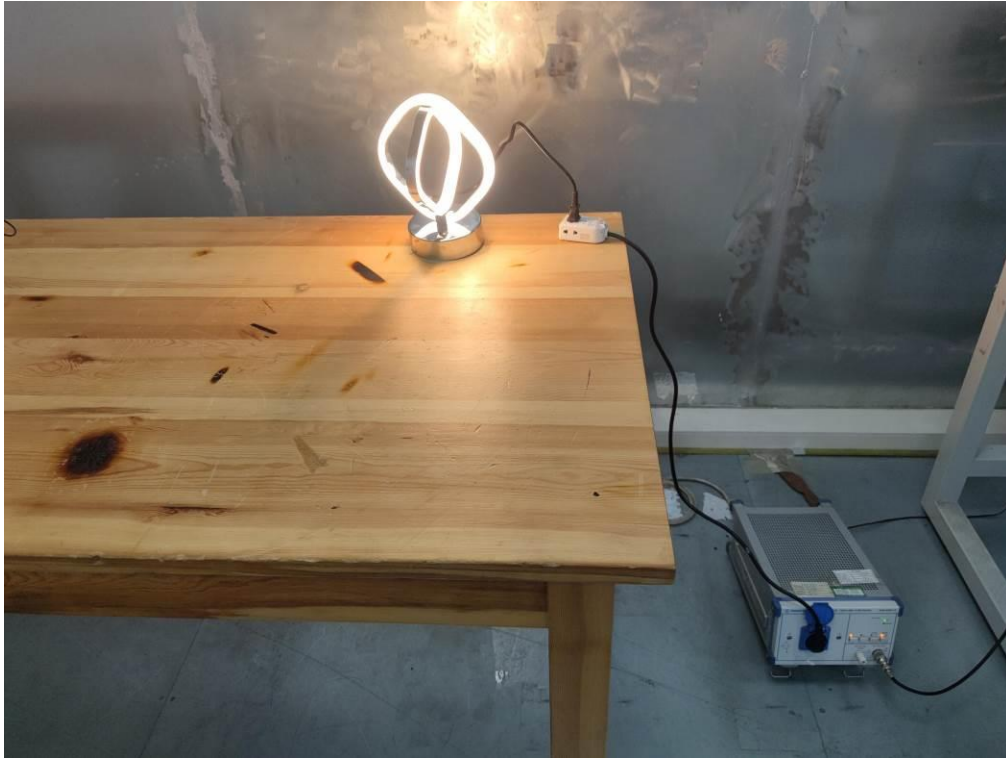
Conducted Emission-AC adapter charge mode
