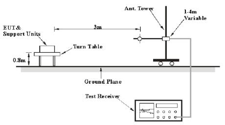
The radiated emission were performed in the 3 meters chamber test site, using the setup accordance with the ANSI C63.4-2014. The specification used was with the FCC Part 15 B Class B limits.
