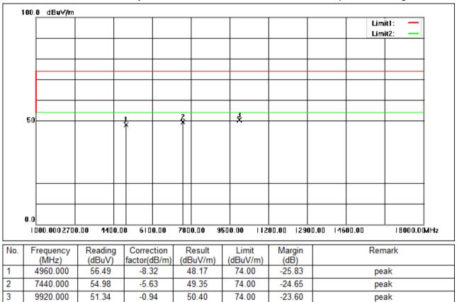
Test Mode: 00; Polarity: Horizontal; Modulation:GFSK; Data Rate:1Mbps; Channel:High
