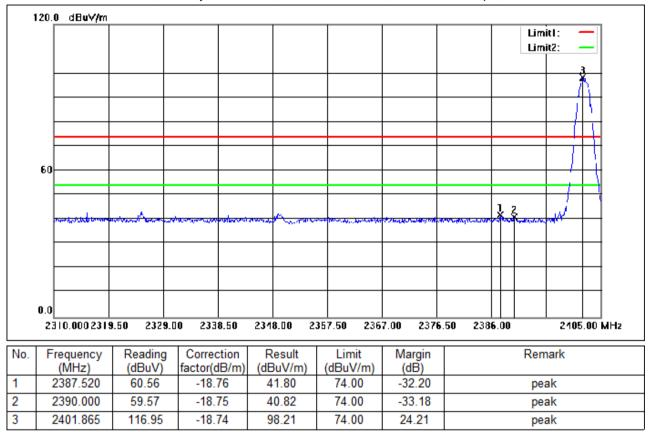
Test Mode: 00; Polarity: Horizontal; Modulation:GFSK; Data Rate:2Mbps; Channel:Low
