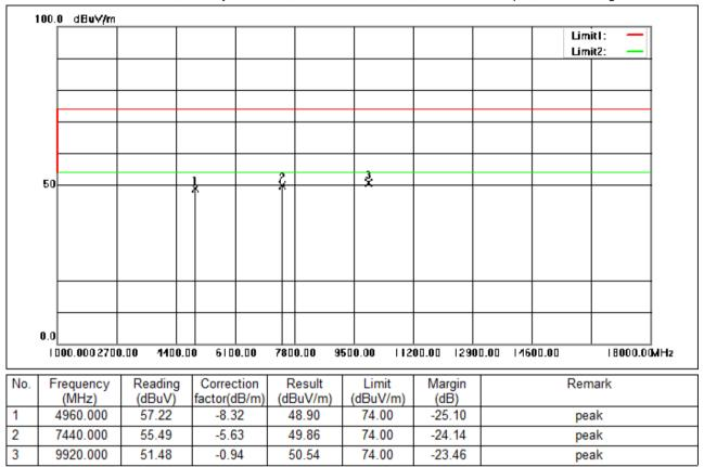
Test Mode: 00; Polarity: Vertical; Modulation:GFSK; Data Rate:1Mbps; Channel:High
