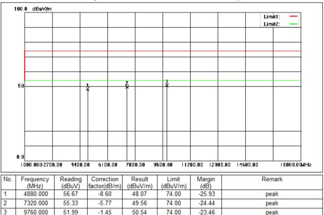
Test Mode: 00; Polarity: Horizontal; Modulation:GFSK; Data Rate:2Mbps; Channel:middle
