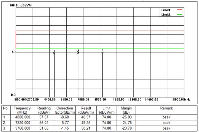
Test Mode: 00; Polarity: Vertical; Modulation:GFSK; Data Rate:1Mbps; Channel:middle
