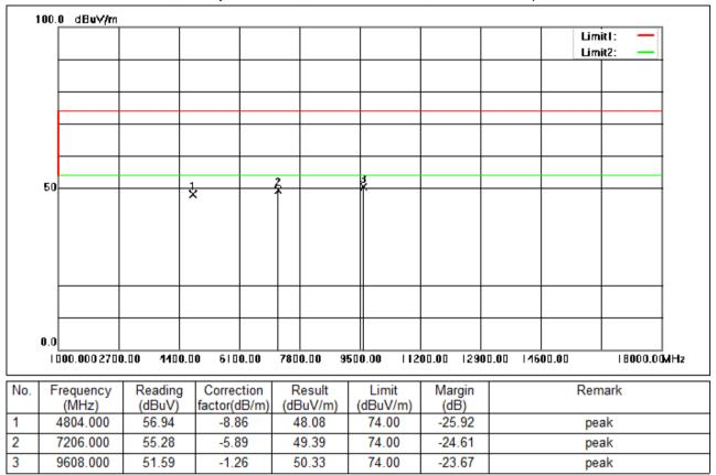
Test Mode: 00; Polarity: Horizontal; Modulation:GFSK; Data Rate:1Mbps; Channel:Low
