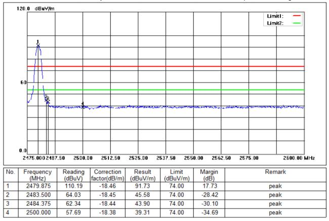
Test Mode: 00; Polarity: Horizontal; Modulation:GFSK; Data Rate:2Mbps; Channel:High
