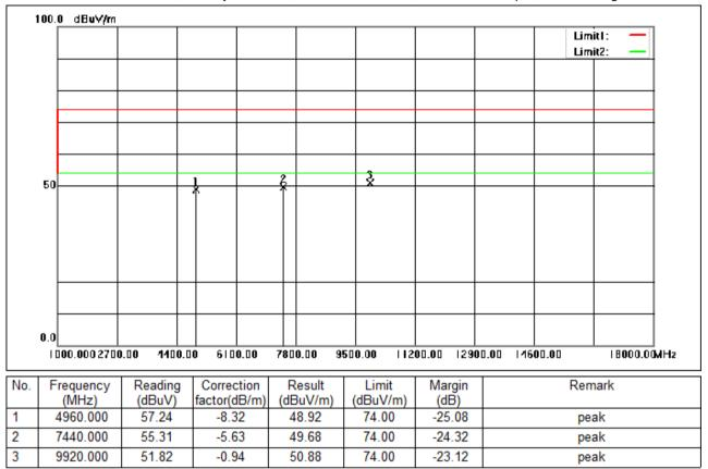
Test Mode: 00; Polarity: Vertical; Modulation:GFSK; Data Rate:2Mbps; Channel:High
