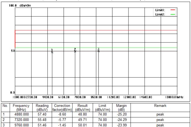
Test Mode: 00; Polarity: Horizontal; Modulation:GFSK; Data Rate:1Mbps; Channel:middle
