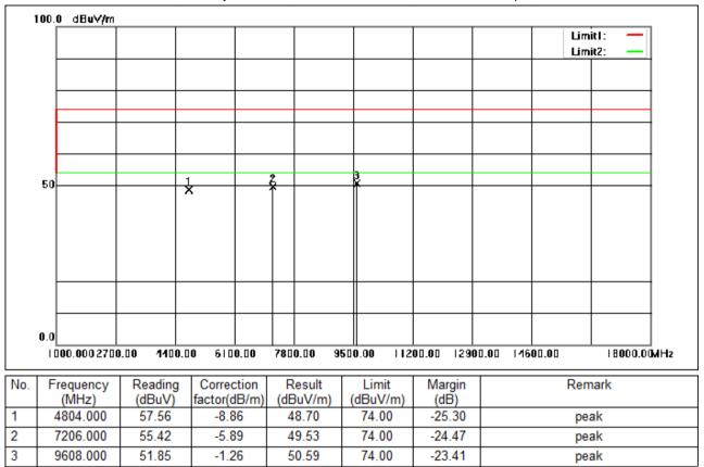
Test Mode: 00; Polarity: Vertical; Modulation:GFSK; Data Rate:2Mbps; Channel:Low
