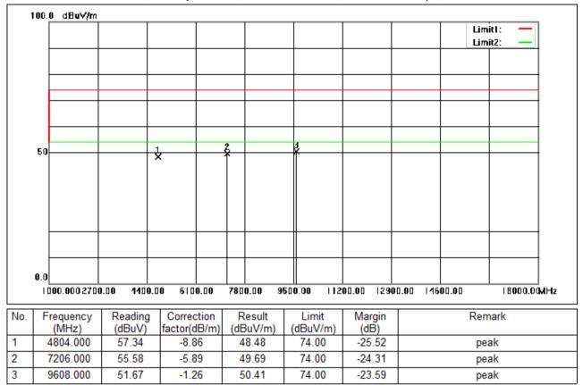
Test Mode: 00; Polarity: Vertical; Modulation:GFSK; Data Rate:1Mbps; Channel:Low
