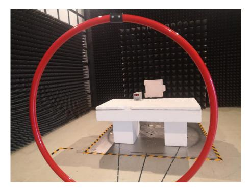
Radiated Emissions (9kHz - 30MHz)
