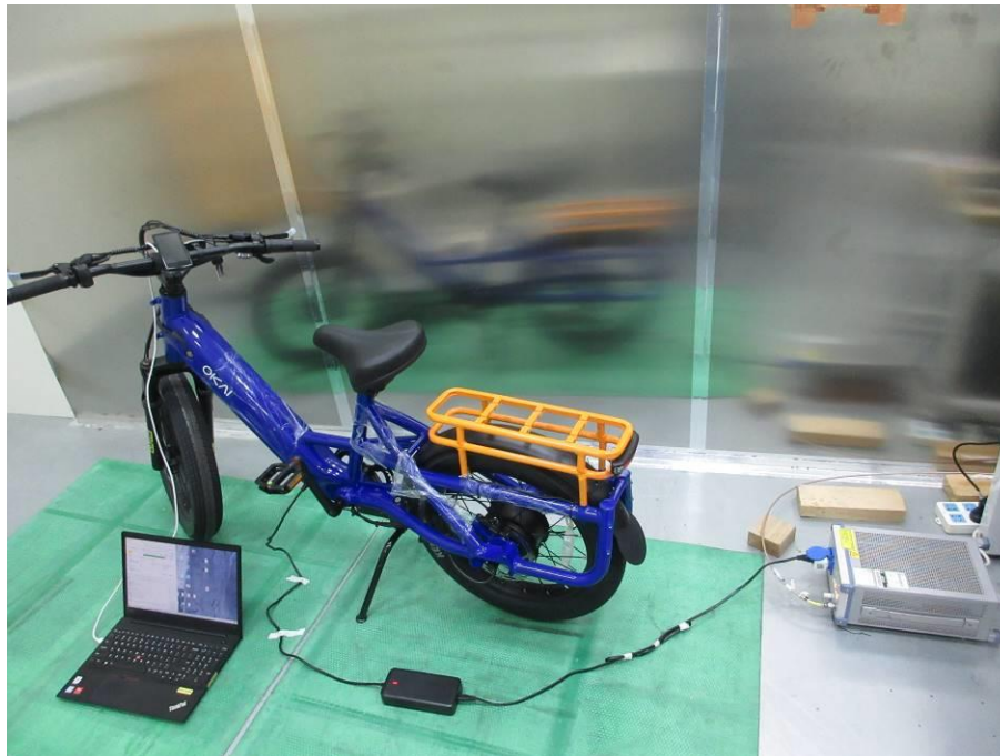
POWERLINE CONDUCTED EMISSIONS MEASUREMENT SETUP
