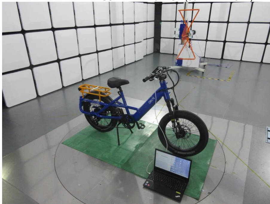
RADIATED RF MEASUREMENT SETUP (30MHz ~ 1 GHz)
