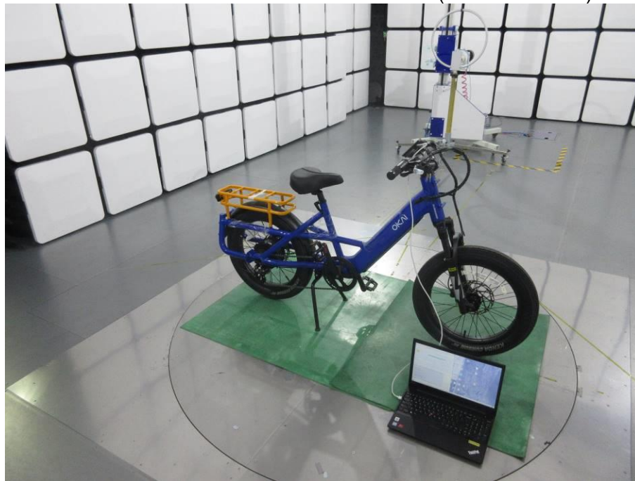
RADIATED RF MEASUREMENT SETUP (9kHz ~ 30 MHz)
