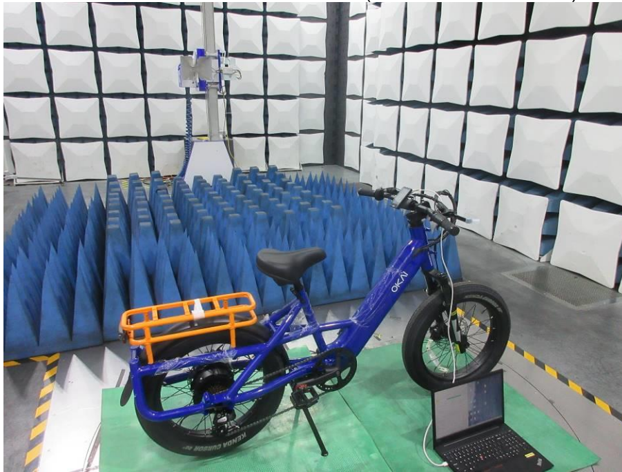
RADIATED RF MEASUREMENT SETUP (ABOVE 1 GHz- X axis) -Part 1
