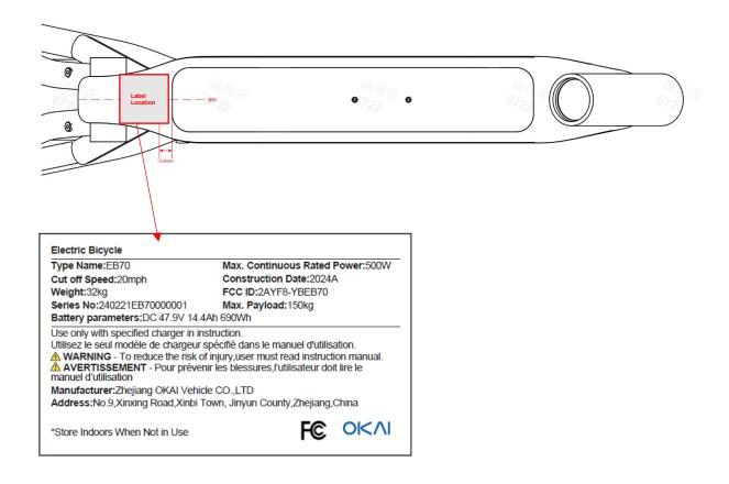
Note: This would be a plastic label with a permanent adhesive bottom of the carframe.
