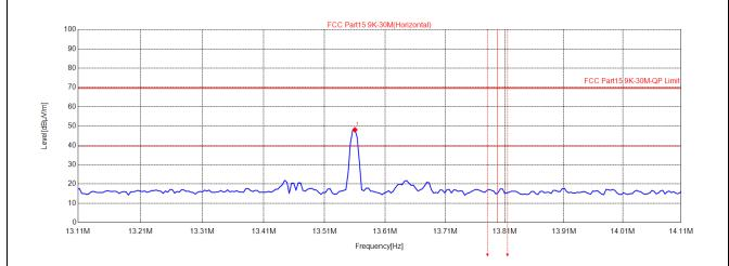
Margin [dB] =Limit [dB $\mu$ V/m] – Level [dB $\mu$ V/m]
