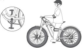
16.Stop pedaling to reduce speed and squeeze brake lever to brake.(Left brake lever controls front wheel braking, right brake lever controls rear wheel braking).
