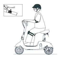
$13.\mbox{Release}$  the acceleration handle to reduce speed, and squeeze the brake lever to brake.
