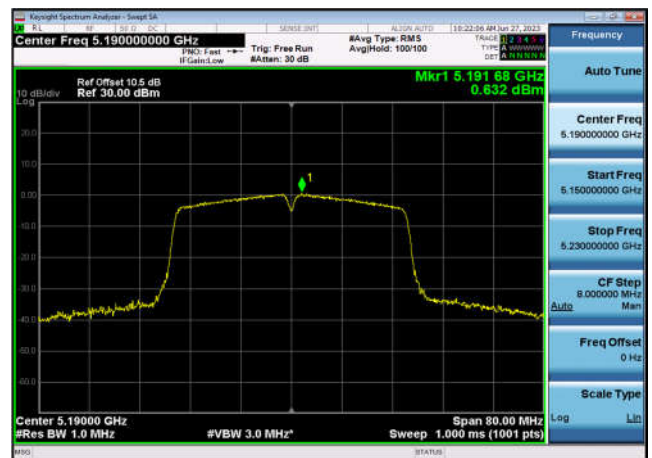
U-NII-1 Power spectral density-802.11 ac(40MHz),5190MHz,Ant1
