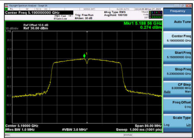
U-NII-1 Power spectral density-802.11 a(20MHz),5180MHz,Ant1
