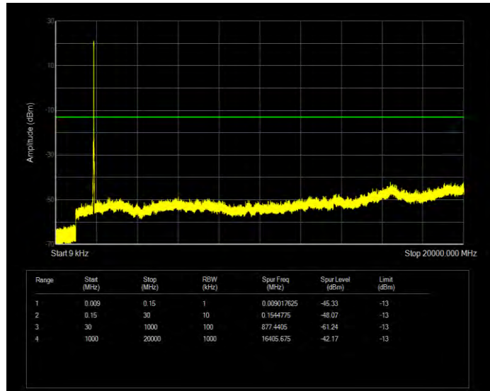
Band25 QPSK BW=10MHz Channel=26640 RB Size=50 Position=#0
