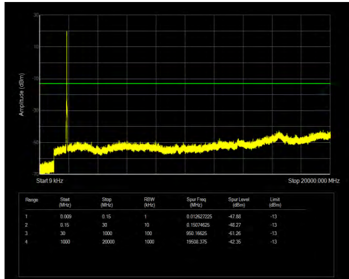
Band25 QPSK BW=15MHz Channel=26615 RB Size=75 Position=#0
