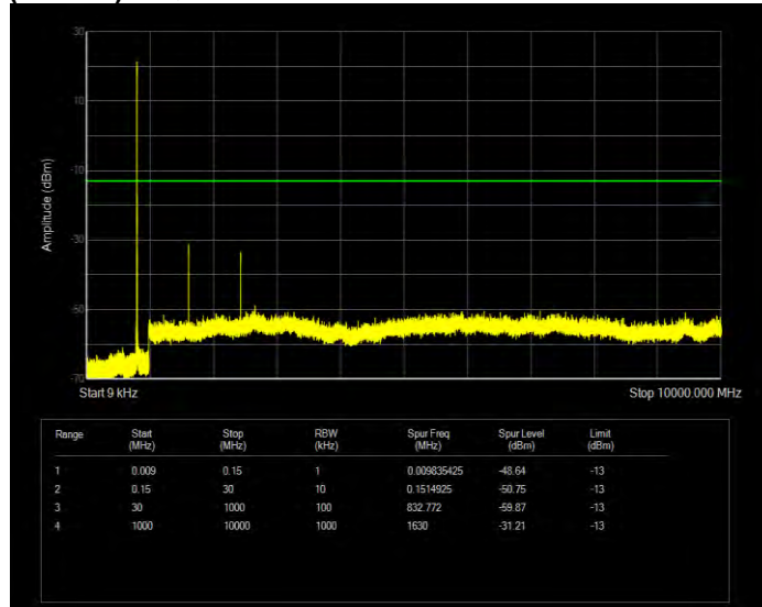
Band26(814-824) 16QAM BW=1.4MHz Channel=26740 RB Size=6 Position=#0
