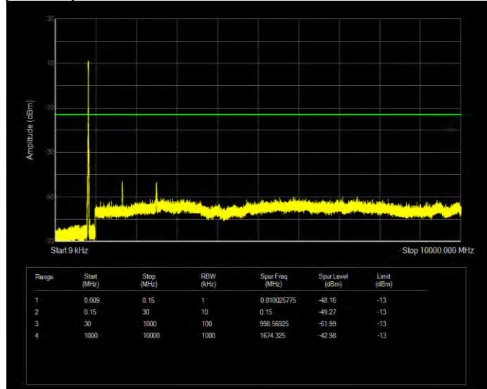
Band26(824-849) 16QAM BW=10MHz Channel=26990 RB Size=50 Position=#0
