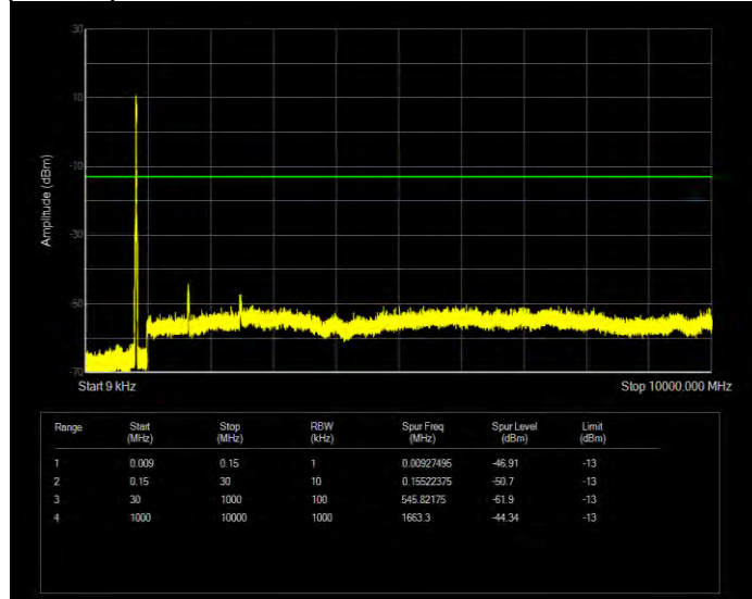
Band26(824-849) 16QAM BW=15MHz Channel=26915 RB Size=75 Position=#0
