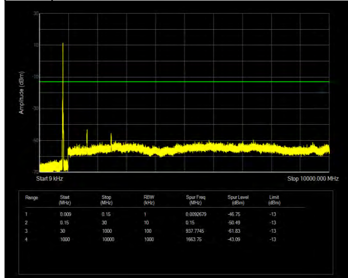
Band26(824-849) 16QAM BW=10MHz Channel=26915 RB Size=50 Position=#0
