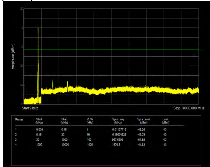
Band26(824-849) 16QAM BW=15MHz Channel=26965 RB Size=75 Position=#0
