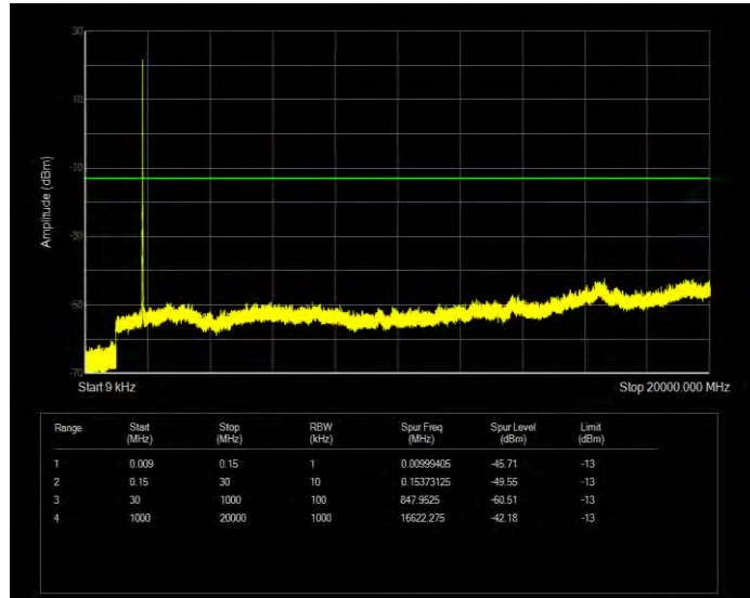
Band25 QPSK BW=5MHz Channel=26365 RB Size=25 Position=#0
