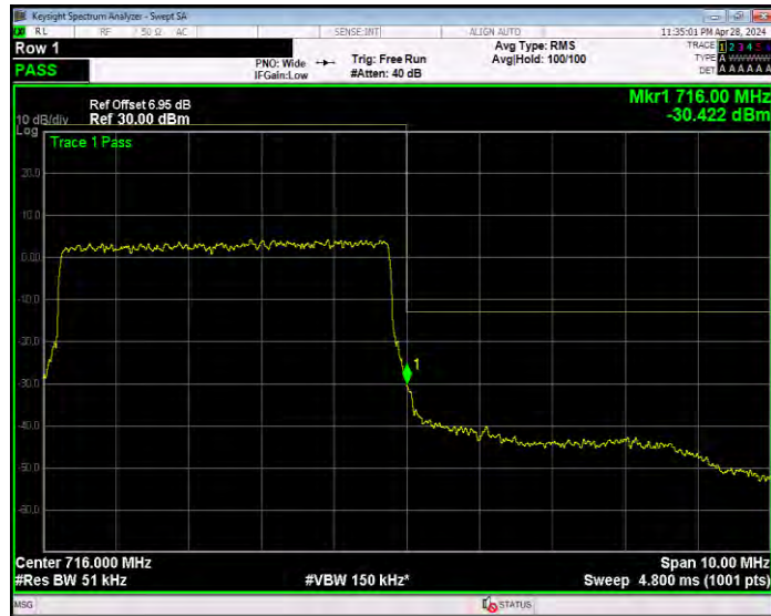
Band25 16QAM BW=1.4MHz Channel=26047 RB Size=6 Position=#0
