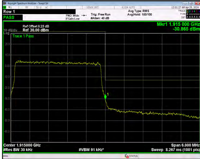
Band25 QPSK BW=5MHz Channel=26065 RB Size=25 Position=#0
