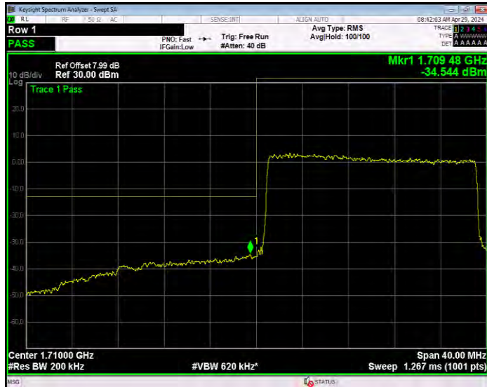
Band66 16QAM BW=20MHz Channel=132572 RB Size=1 Position=#0
