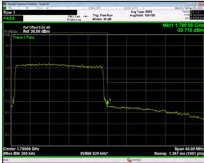
Band66 16QAM BW=3MHz Channel=131987 RB Size=1 Position=#0
