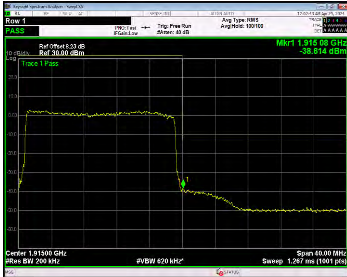
Band25 16QAM BW=3MHz Channel=26055 RB Size=15 Position=#0
