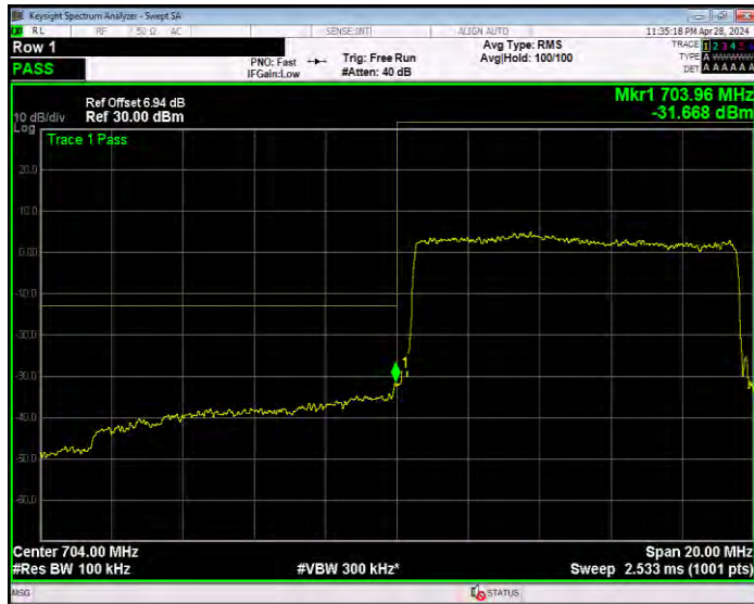
Band17 QPSK BW=10MHz Channel=23800 RB Size=1 Position=#0
