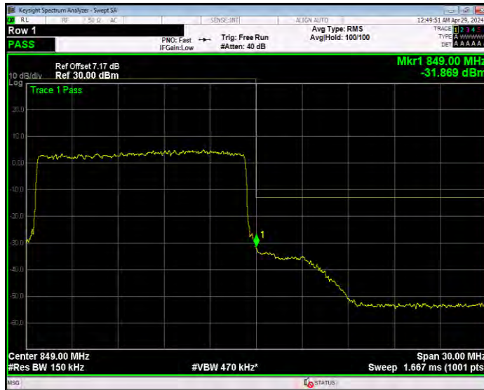
Band26(824-849) QPSK BW=3MHz Channel=26805 RB Size=15 Position=#0
