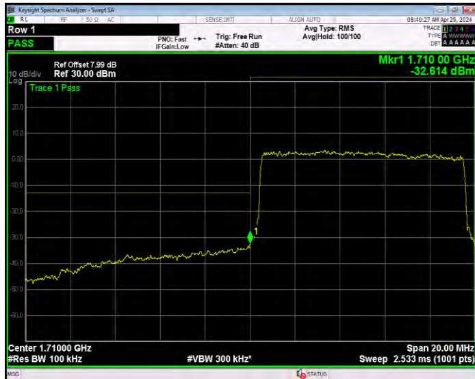
Band66 16QAM BW=10MHz Channel=132622 RB Size=1 Position=#0
