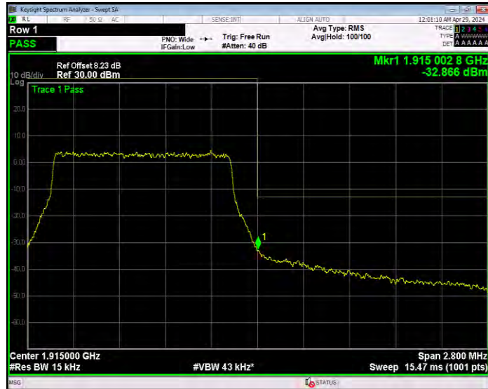
Band25 16QAM BW=10MHz Channel=26090 RB Size=50 Position=#0
