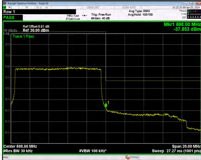
Band71 QPSK BW=15MHz Channel=133197 RB Size=1 Position=#0
