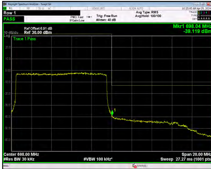
Band71 16QAM BW=15MHz Channel=133197 RB Size=1 Position=#0
