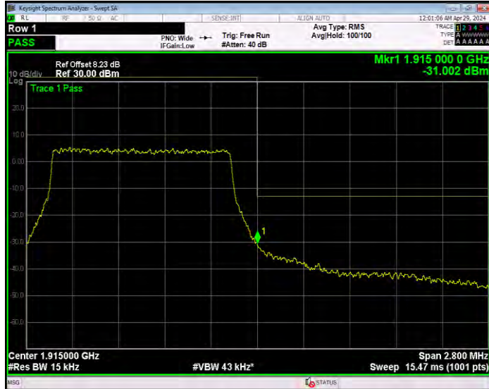
Band25 QPSK BW=10MHz Channel=26090 RB Size=50 Position=#0
