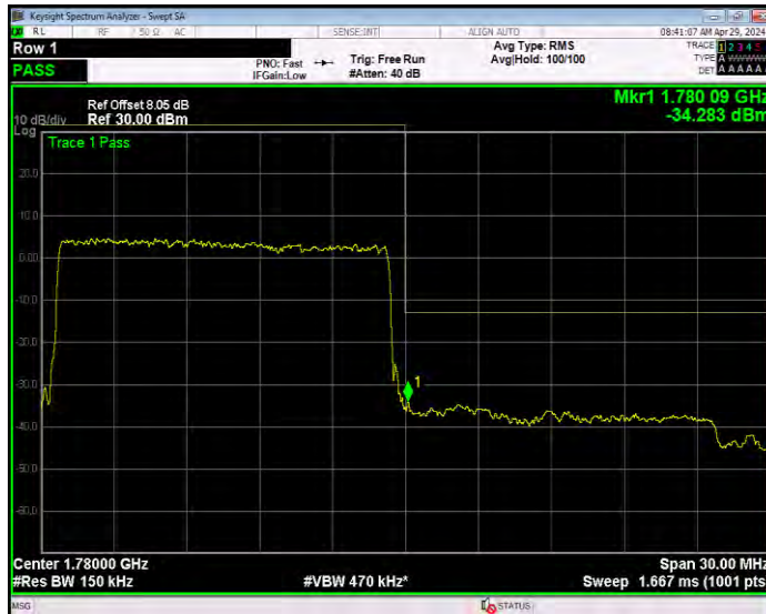
Band66 QPSK BW=20MHz Channel=132072 RB Size=1 Position=#0
