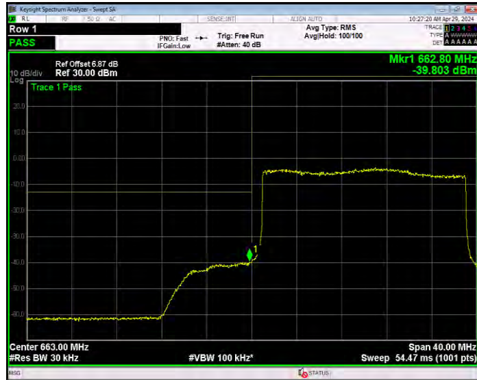
Band71 16QAM BW=20MHz Channel=133372 RB Size=1 Position=#0
