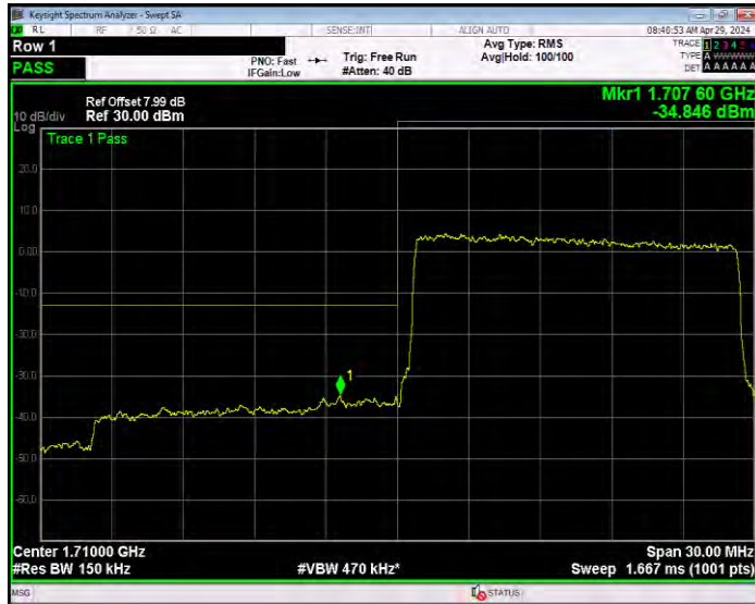
Band66 QPSK BW=15MHz Channel=132597 RB Size=1 Position=#0
