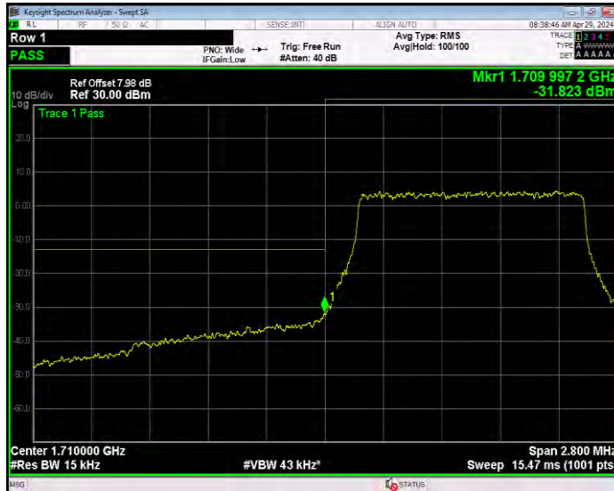
Band66 16QAM BW=1.4MHz Channel=132665 RB Size=1 Position=#0
