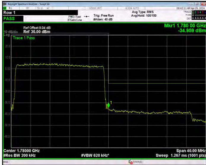
Band66 QPSK BW=3MHz Channel=131987 RB Size=1 Position=#0
