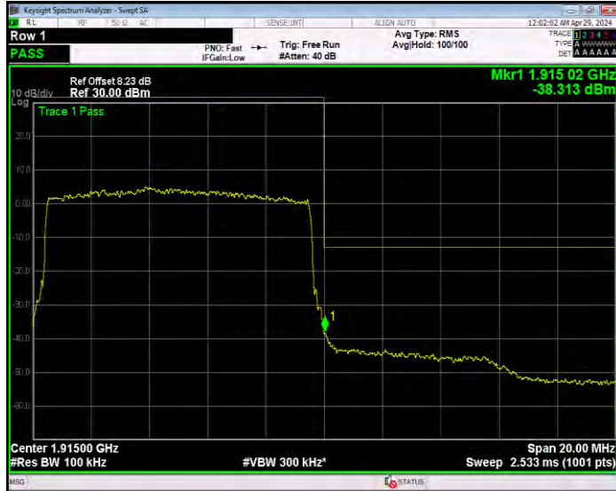
Band25 QPSK BW=15MHz Channel=26115 RB Size=75 Position=#0
