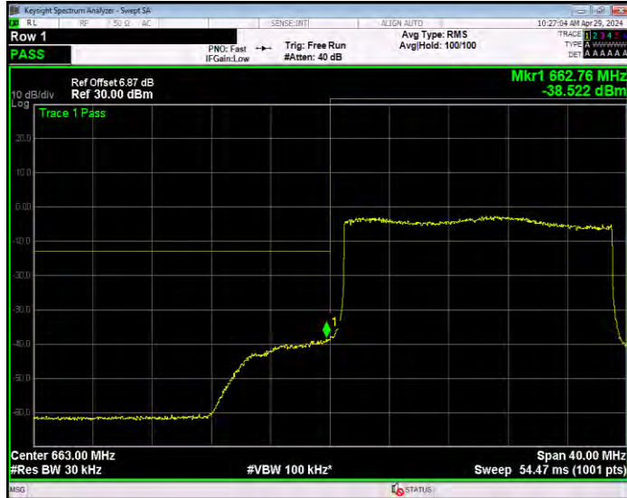
Band71 QPSK BW=20MHz Channel=133372 RB Size=1 Position=#0
