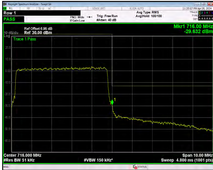
Band17 QPSK BW=10MHz Channel=23780 RB Size=1 Position=#0
