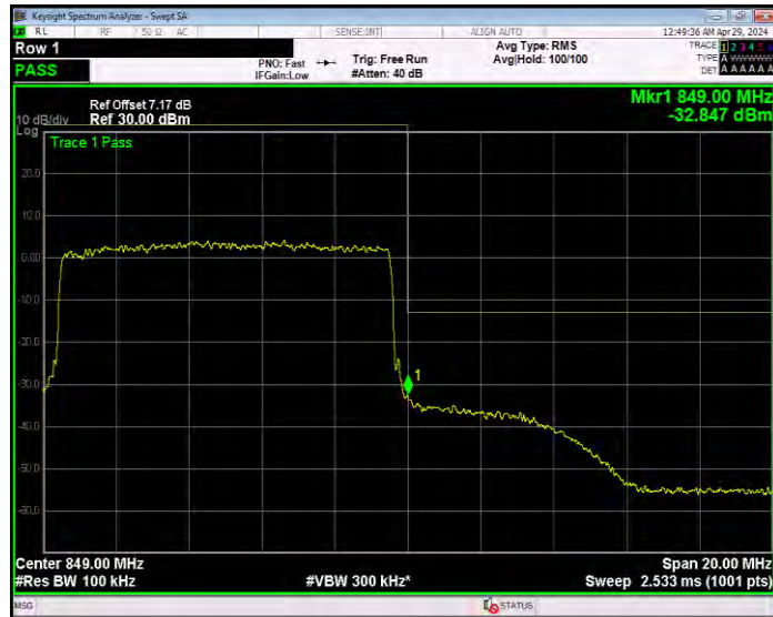
Band26(824-849) 16QAM BW=15MHz Channel=26865 RB Size=75 Position=#0
