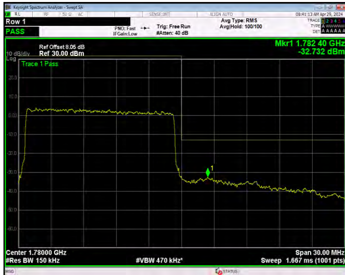
Band66 16QAM BW=20MHz Channel=132072 RB Size=1 Position=#0
