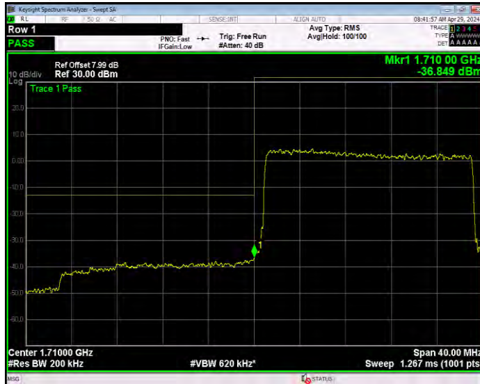
Band66 QPSK BW=20MHz Channel=132572 RB Size=1 Position=#0
