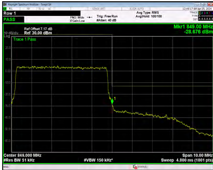
Band26(824-849) QPSK BW=1.4MHz Channel=26797 RB Size=6 Position=#0
