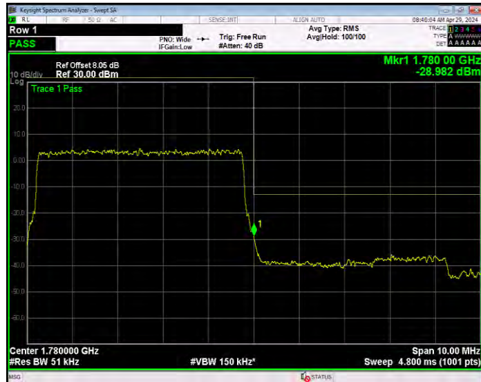
Band71 16QAM BW=10MHz Channel=133172 RB Size=1 Position=#0
