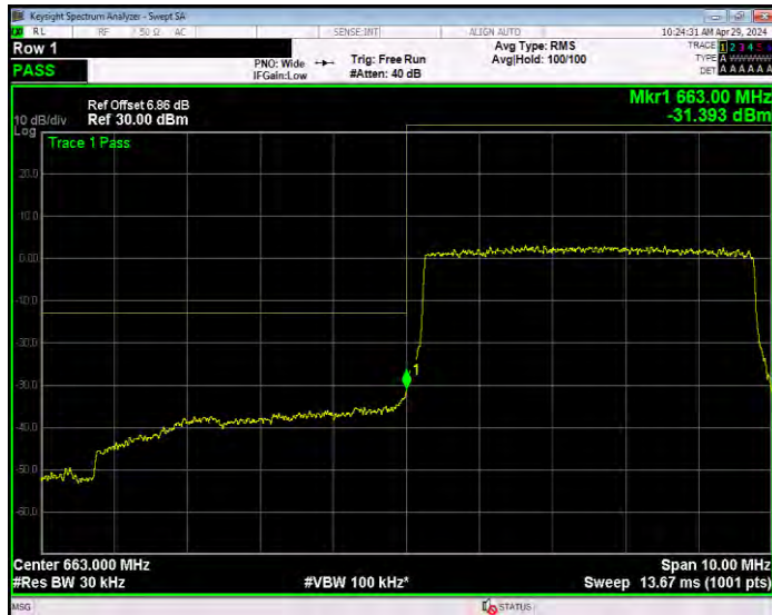
Band71 QPSK BW=5MHz Channel=133447 RB Size=1 Position=#0
