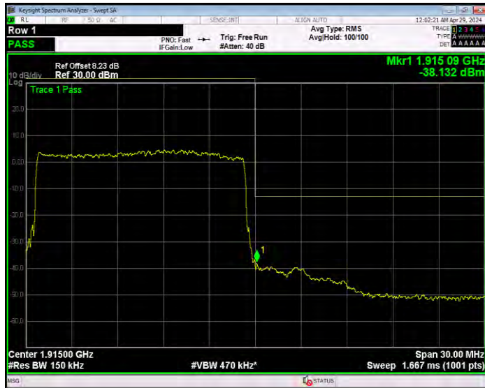
Band25 QPSK BW=20MHz Channel=26140 RB Size=100 Position=#0
