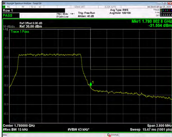
Band66 16QAM BW=10MHz Channel=132022 RB Size=1 Position=#0
