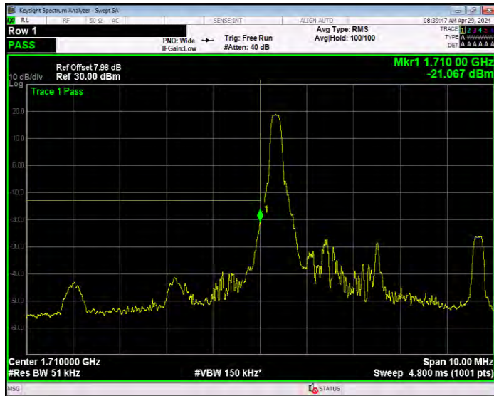
Band66 QPSK BW=5MHz Channel=131997 RB Size=25 Position=#0
