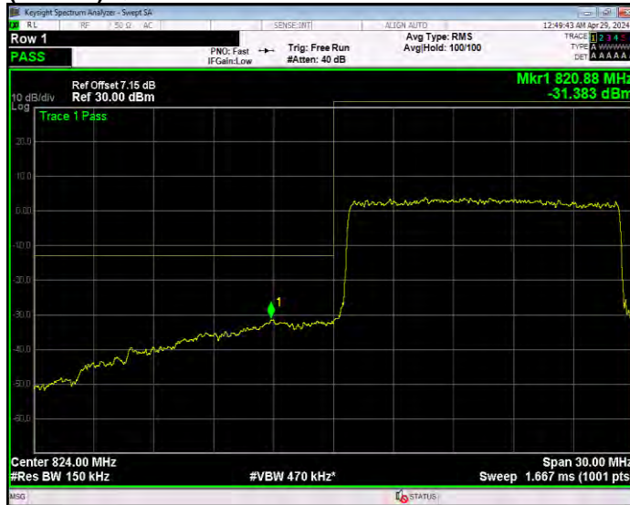
Band26(824-849) QPSK BW=15MHz Channel=26965 RB Size=75 Position=#0
