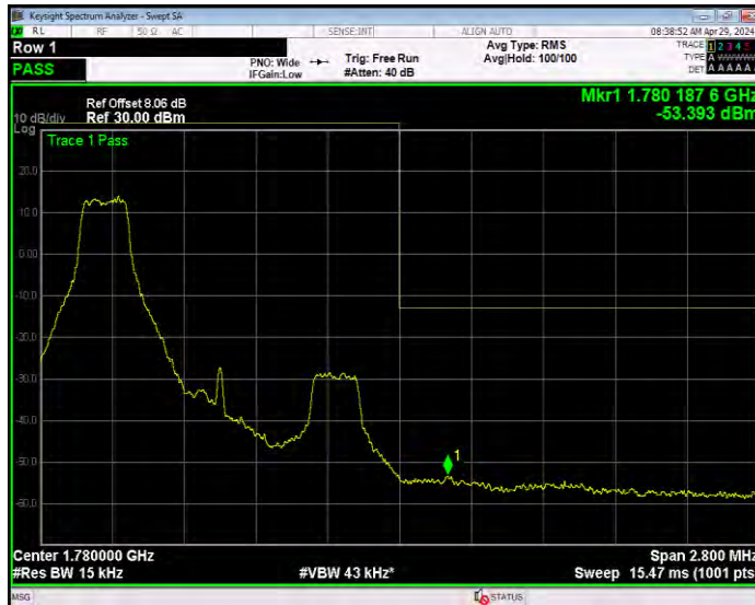
Band66 QPSK BW=1.4MHz Channel=132665 RB Size=6 Position=#0
