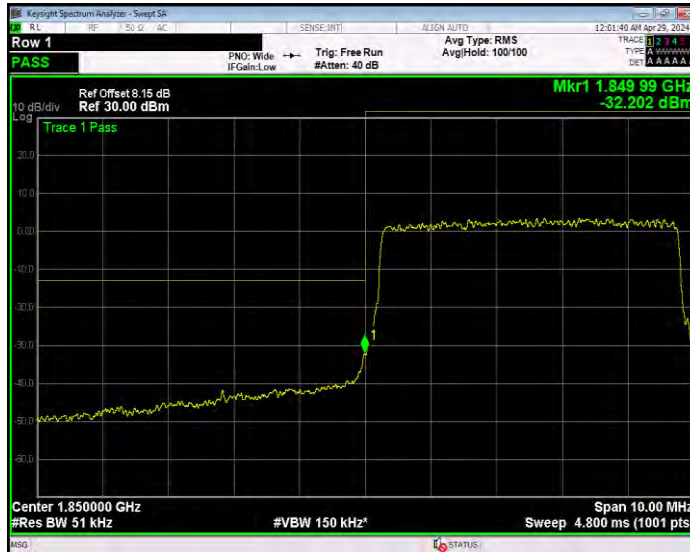
Band25 16QAM BW=5MHz Channel=26665 RB Size=25 Position=#0
