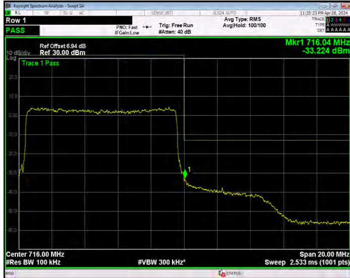
Band17 QPSK BW=5MHz Channel=23755 RB Size=1 Position=#0
