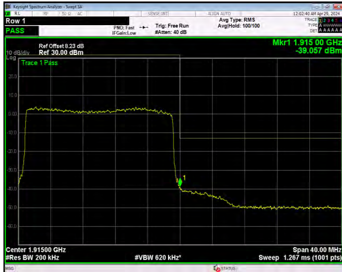
Band25 QPSK BW=3MHz Channel=26055 RB Size=15 Position=#0
