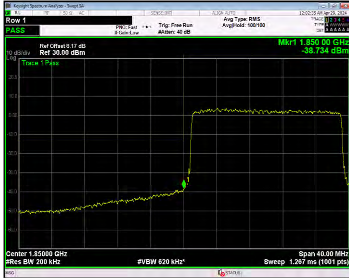
Band25 16QAM BW=20MHz Channel=26590 RB Size=100 Position=#0
