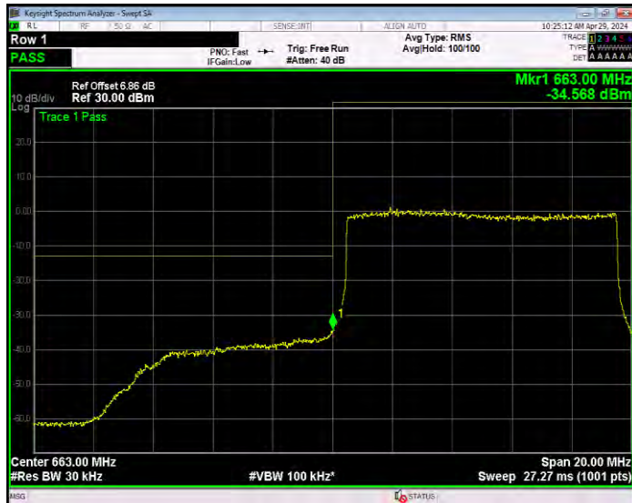
Band71 QPSK BW=10MHz Channel=133422 RB Size=1 Position=#0
