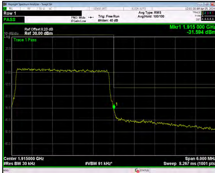
Band25 16QAM BW=5MHz Channel=26065 RB Size=25 Position=#0
