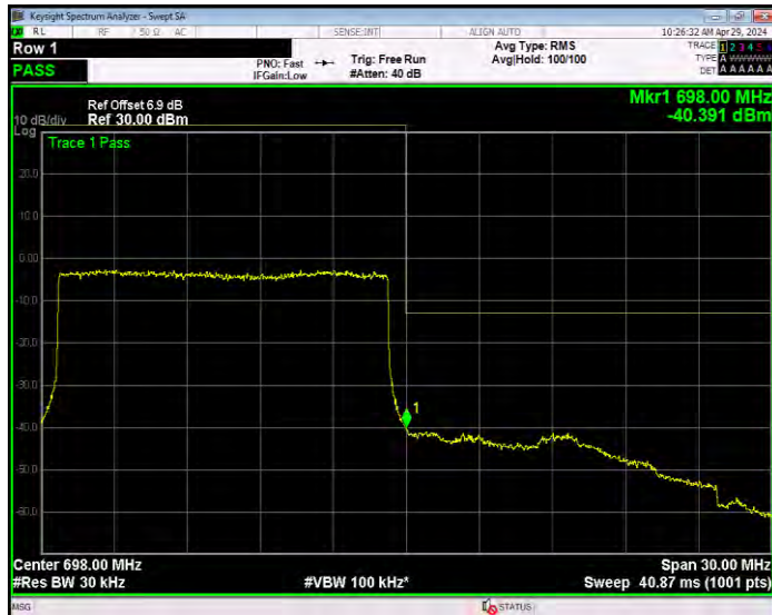
Band71 QPSK BW=20MHz Channel=133222 RB Size=1 Position=#0
