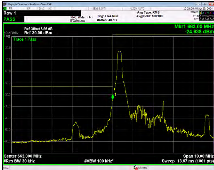
Band71 QPSK BW=5MHz Channel=133147 RB Size=25 Position=#0
