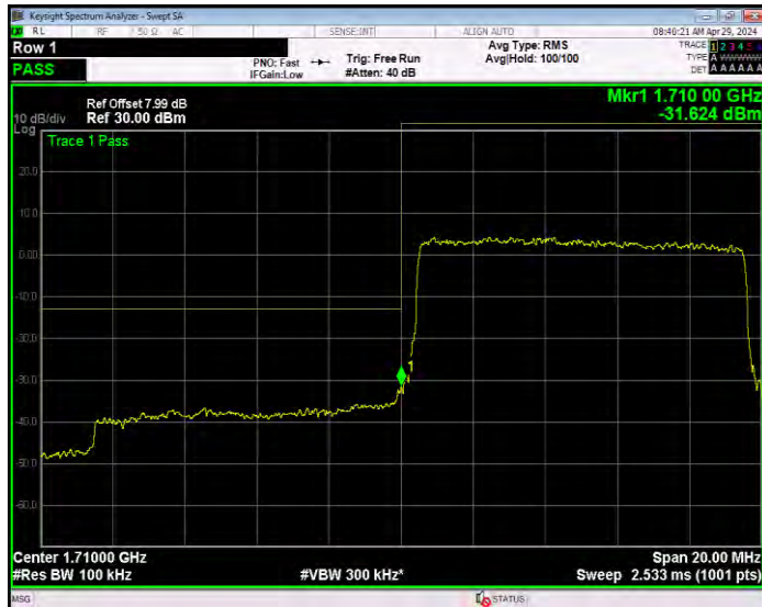
Band66 QPSK BW=10MHz Channel=132622 RB Size=1 Position=#0
