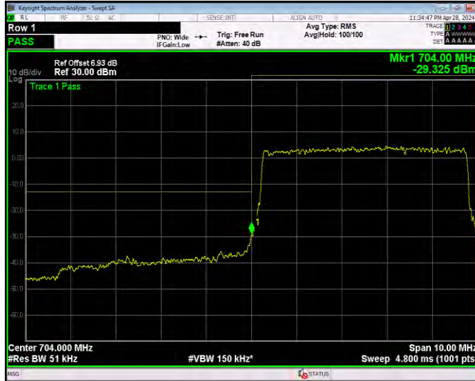
Band17 QPSK BW=5MHz Channel=23825 RB Size=1 Position=#0
