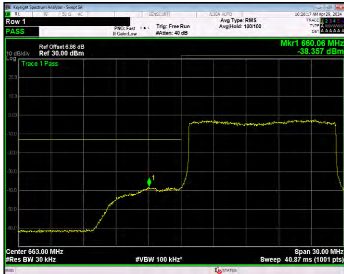
Band71 16QAM BW=15MHz Channel=133397 RB Size=1 Position=#0
