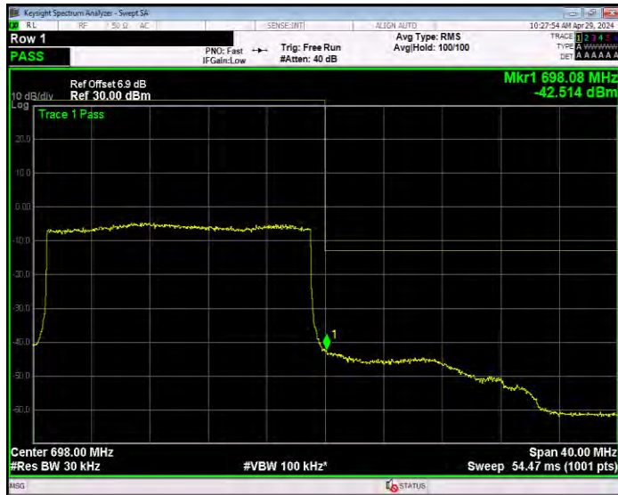
Band71 16QAM BW=5MHz Channel=133147 RB Size=1 Position=#0
