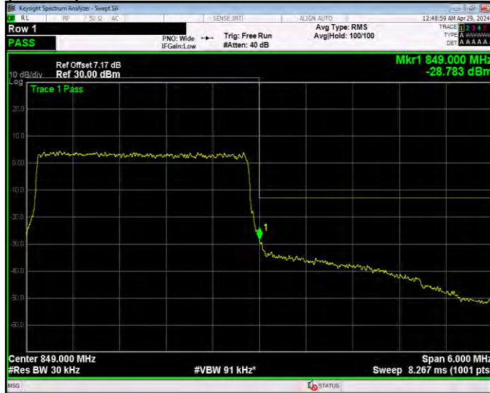
Band26(824-849) 16QAM BW=5MHz Channel=26815 RB Size=25 Position=#0
