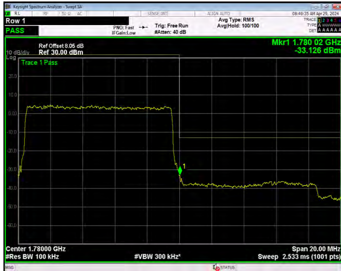
Band66 QPSK BW=15MHz Channel=132047 RB Size=1 Position=#0
