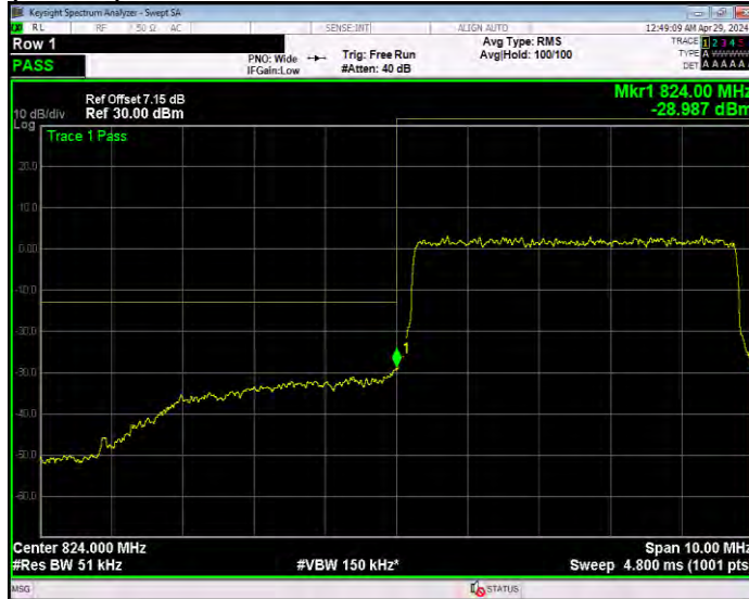
Band26(824-849) 16QAM BW=5MHz Channel=27015 RB Size=25 Position=#0
