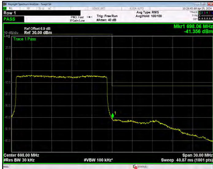
Band71 16QAM BW=20MHz Channel=133222 RB Size=1 Position=#0
