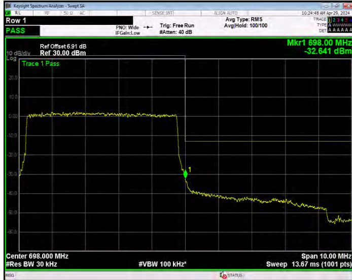
Band71 QPSK BW=5MHz Channel=133447 RB Size=25 Position=#0
