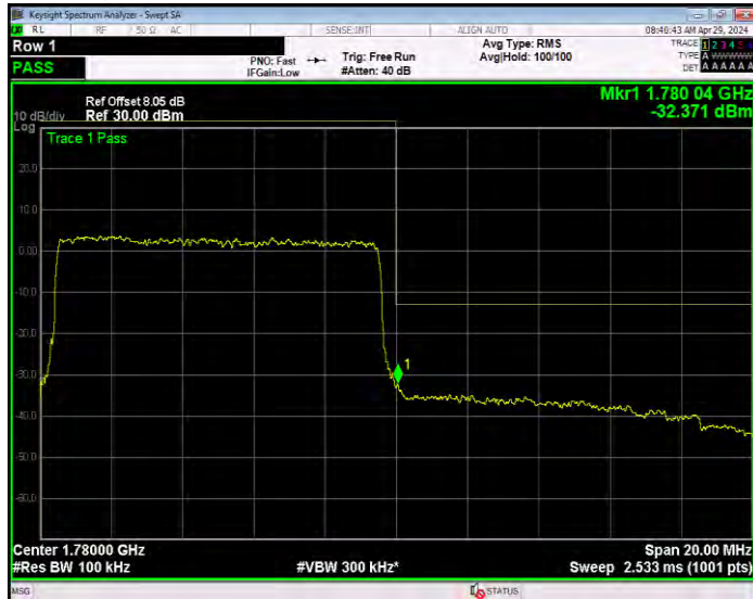
Band66 16QAM BW=15MHz Channel=132047 RB Size=1 Position=#0
