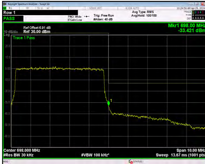
Band71 QPSK BW=10MHz Channel=133172 RB Size=1 Position=#0
