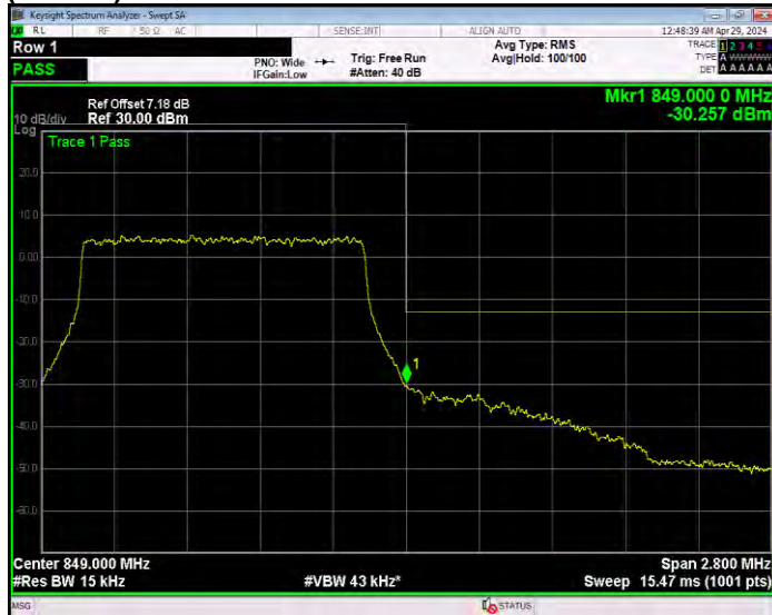
Band26(824-849) 16QAM BW=10MHz Channel=26840 RB Size=50 Position=#0
