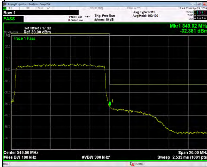
Band26(824-849) QPSK BW=15MHz Channel=26865 RB Size=75 Position=#0
