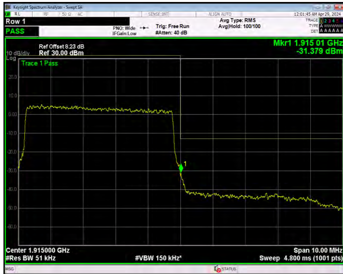
Band26(814-824) 16QAM BW=1.4MHz Channel=26697 RB Size=6 Position=#0
