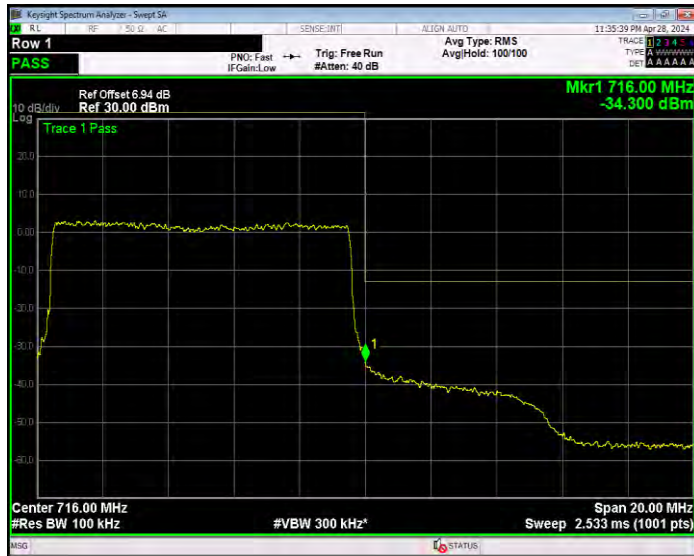
Band17 16QAM BW=5MHz Channel=23755 RB Size=1 Position=#0
