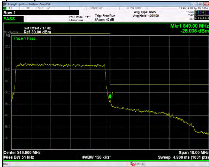
Band41 16QAM BW=10MHz Channel=39700 RB Size=1 Position=#0
