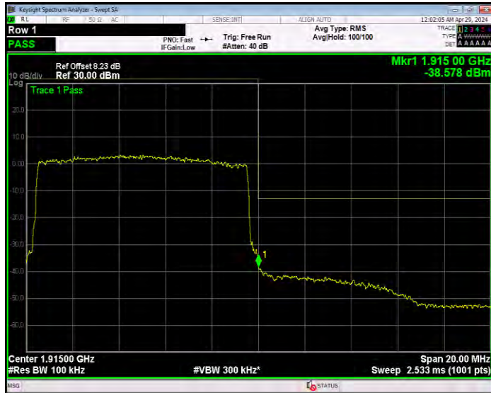
Band25 16QAM BW=15MHz Channel=26115 RB Size=75 Position=#0
