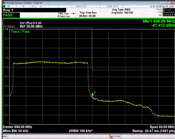
Band71 QPSK BW=5MHz Channel=133147 RB Size=1 Position=#0
