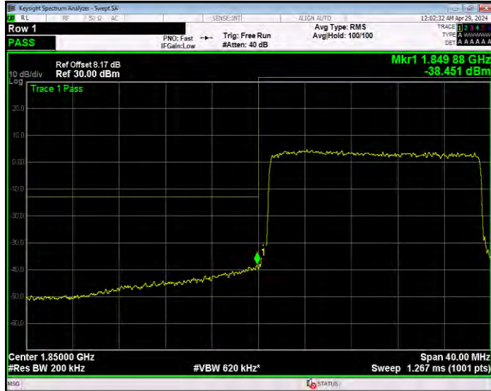
Band25 QPSK BW=20MHz Channel=26590 RB Size=100 Position=#0
