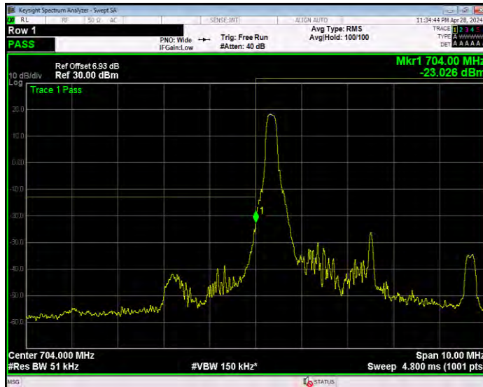
Band17 QPSK BW=5MHz Channel=23755 RB Size=25 Position=#0
