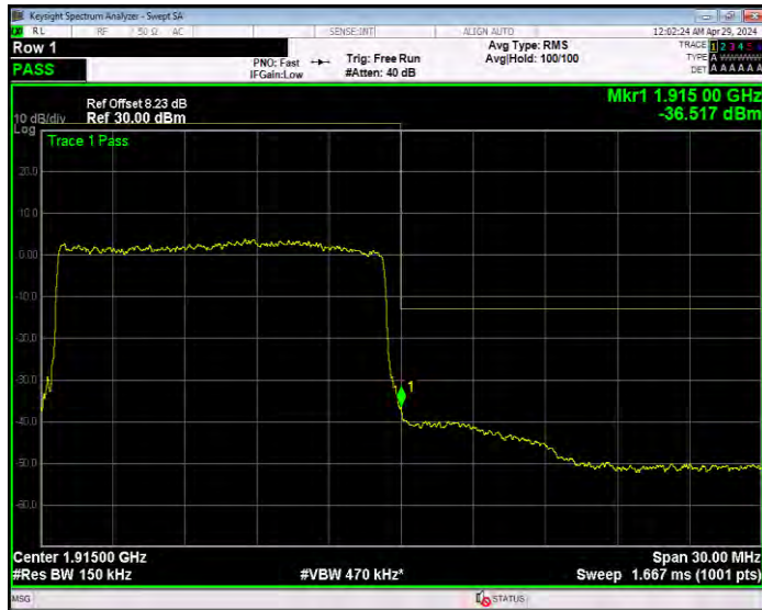
Band25 16QAM BW=20MHz Channel=26140 RB Size=100 Position=#0
