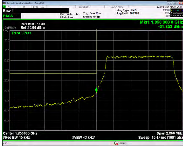
Band25 QPSK BW=1.4MHz Channel=26683 RB Size=6 Position=#0
