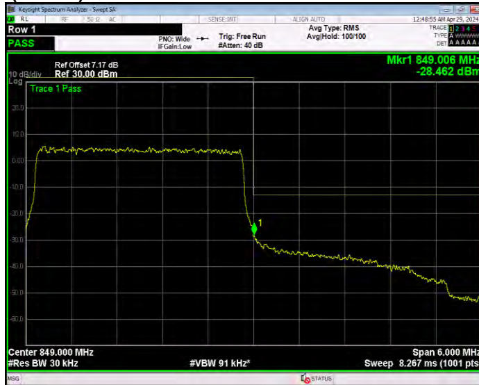
Band26(824-849) QPSK BW=5MHz Channel=26815 RB Size=25 Position=#0
