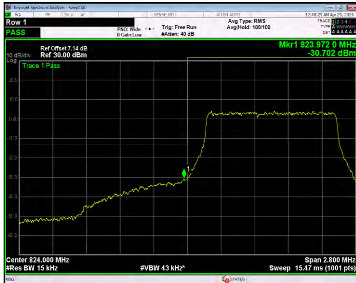
Band26(824-849) 16QAM BW=1.4MHz Channel=27033 RB Size=6 Position=#0
