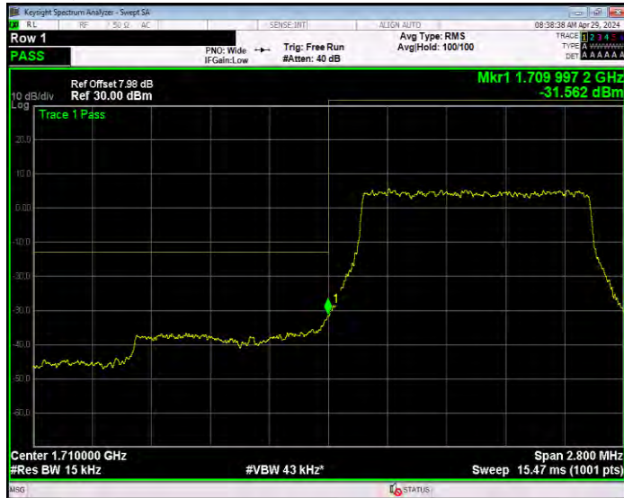
Band66 QPSK BW=1.4MHz Channel=132665 RB Size=1 Position=#0
