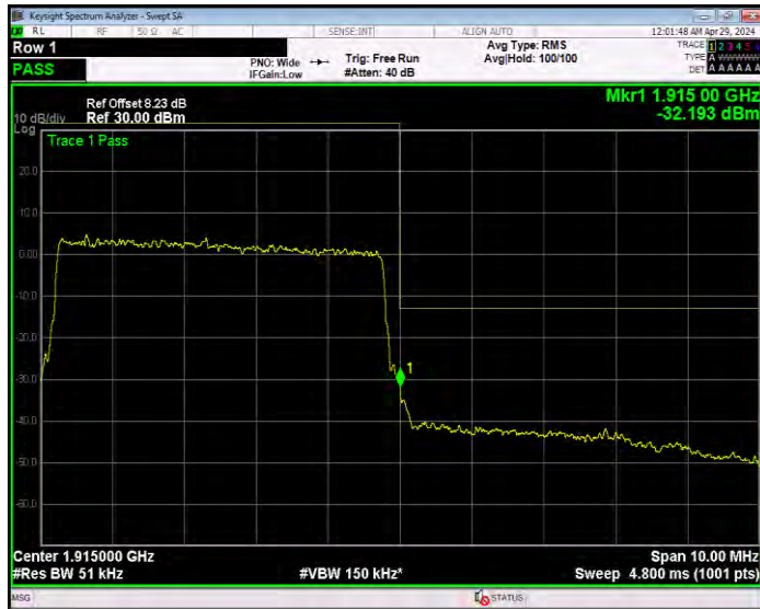
Band25 QPSK BW=1.4MHz Channel=26047 RB Size=6 Position=#0
