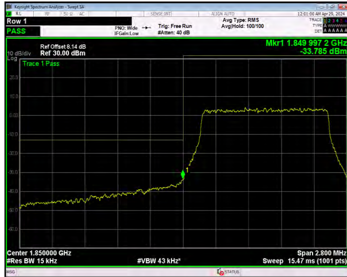
Band25 16QAM BW=1.4MHz Channel=26683 RB Size=6 Position=#0
