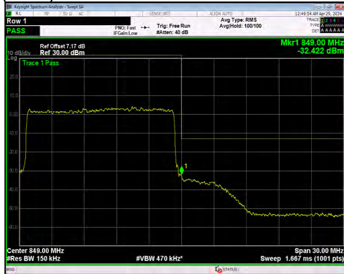
Band26(824-849) 16QAM BW=3MHz Channel=26805 RB Size=15 Position=#0
