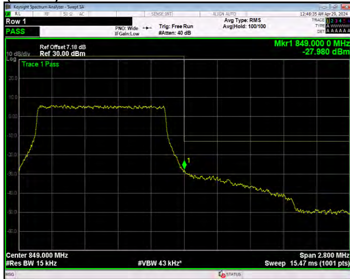
Band26(824-849) QPSK BW=10MHz Channel=26840 RB Size=50 Position=#0
