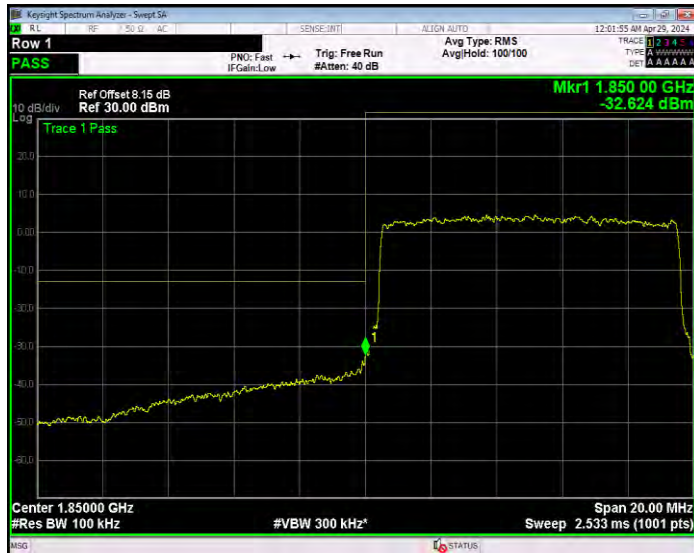
Band25 QPSK BW=10MHz Channel=26640 RB Size=50 Position=#0
