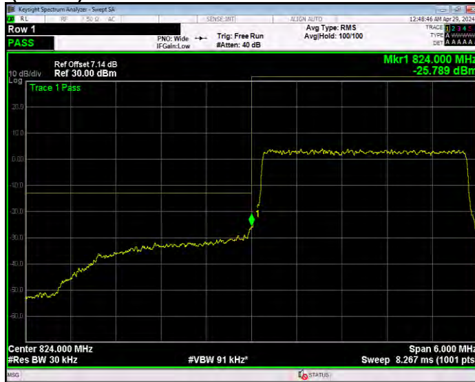
Band26(824-849) QPSK BW=3MHz Channel=27025 RB Size=15 Position=#0
