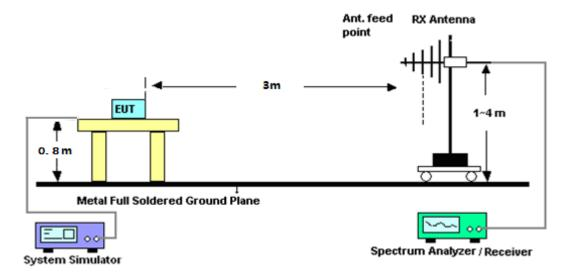
For radiated test from above 1GHz
