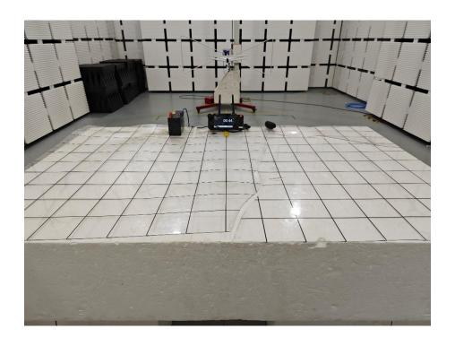
**Set-up for Radiated Spurious Emission, Above 1GHz**
