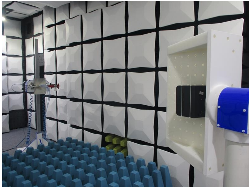
Bild / Picture 7: Test Setup: Radiated Measurements (1 GHz to 25 GHz)
