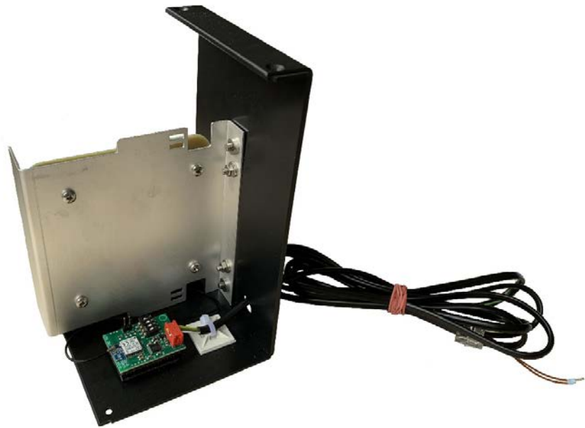
Fig. 10: Connection – beacon 6-pole micro-match connector
