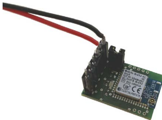
Fig. 13: Connection of beacon in DCT to battery
