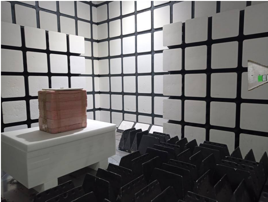
Radiated Emissions View (Above 1 GHz)
