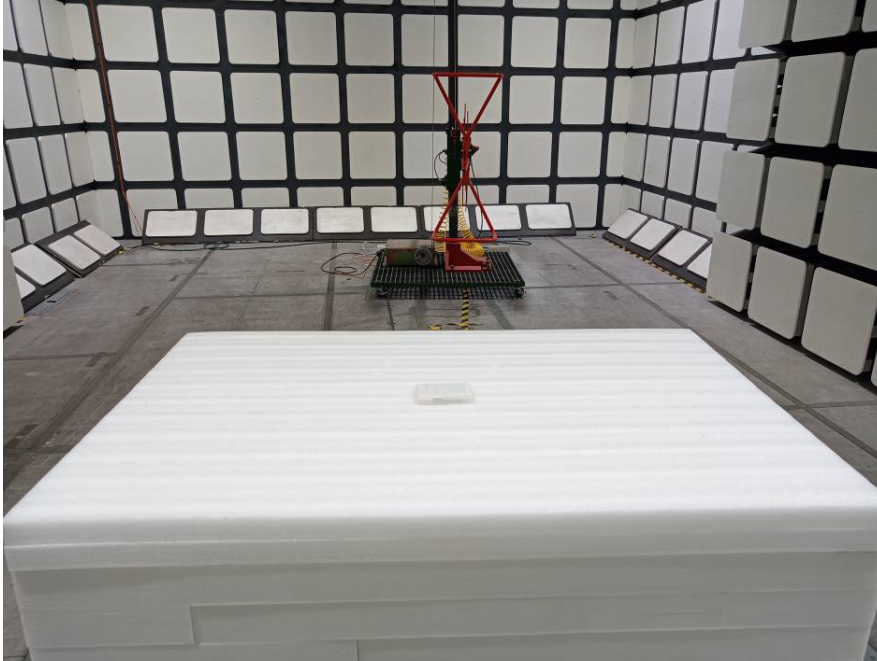
Radiated Emissions View (Below 1 GHz)
