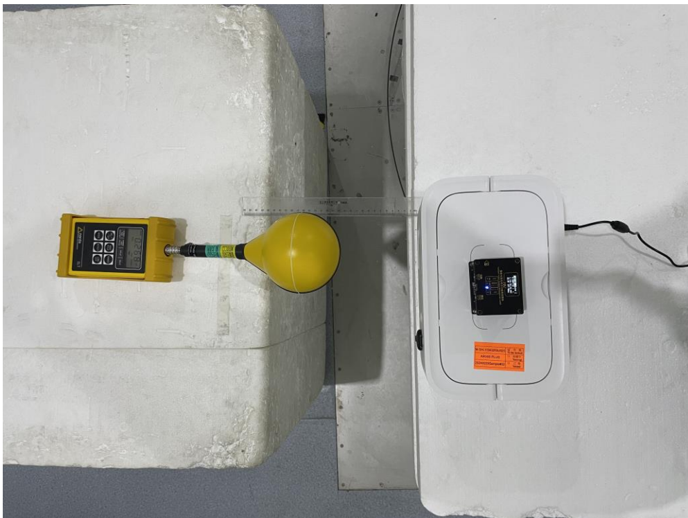
Description: Magnetic Field Emissions Test Setup Mode 2
