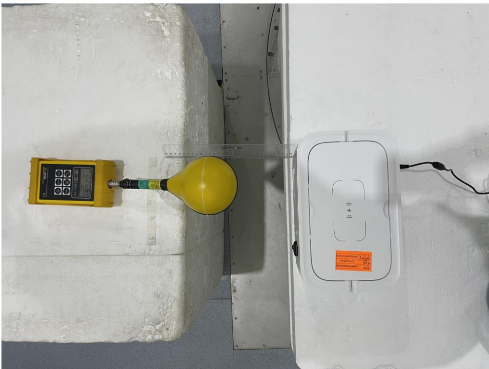
Description: Magnetic Field Emissions Test Setup Mode 1
