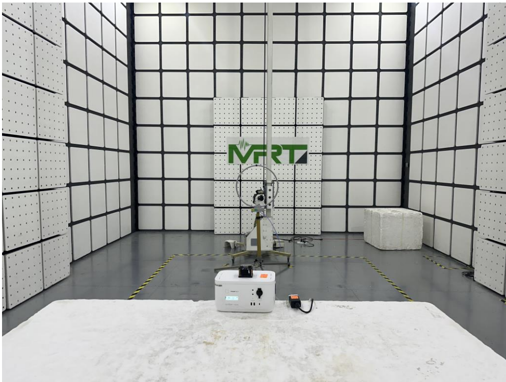
Description: Radiated Emission Test Setup Mode 2
