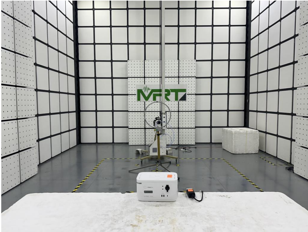
Description: Radiated Emission Test Setup Mode 2
