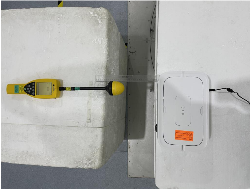
Description: Electric Field Emissions Test Setup Mode 1
