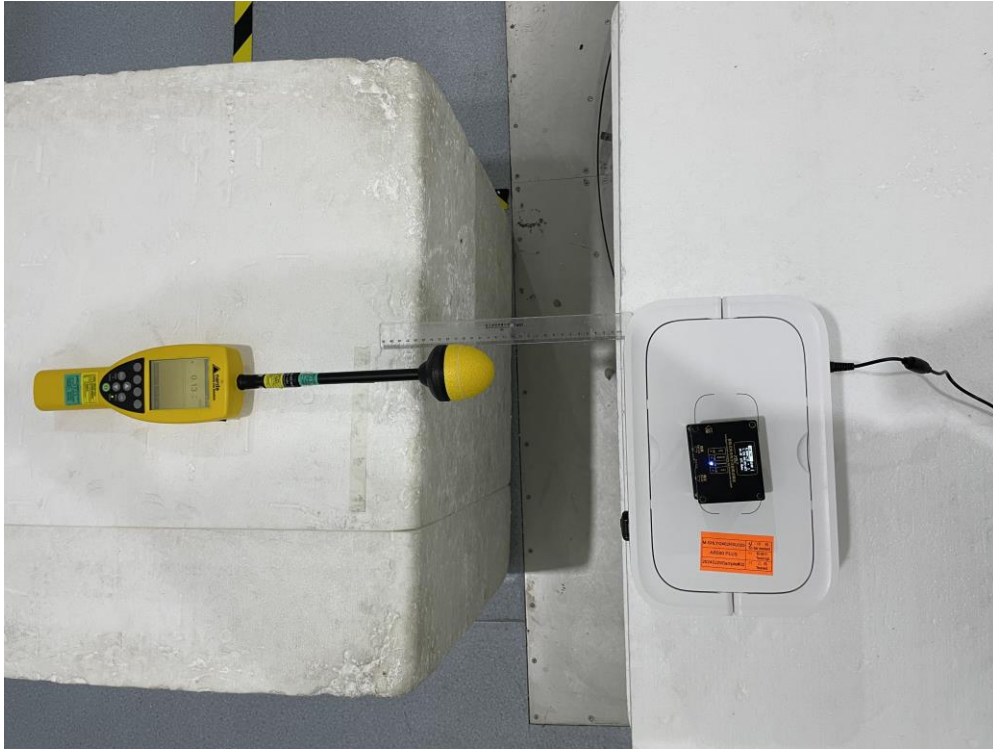
Description: Magnetic Field Emissions Test Setup Mode 2
