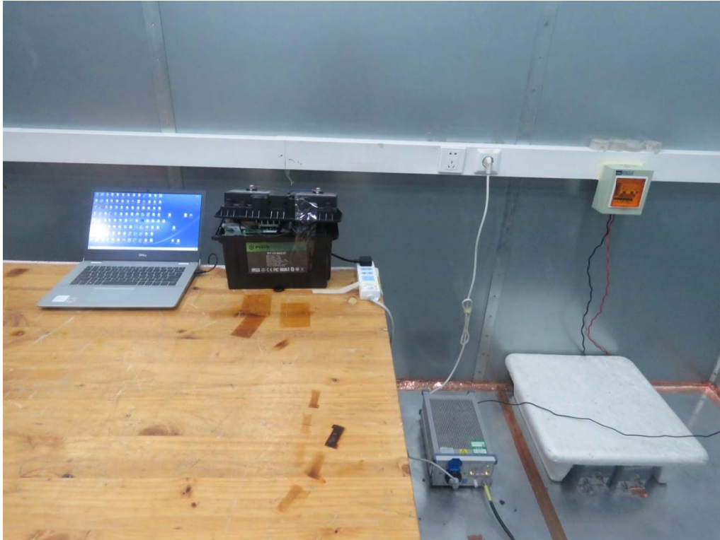
Picture 2 Conducted Emission Test Setup
