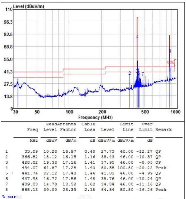
1.Final Level =Receiver Read level + Antenna Factor + Cable Loss – Preamplifier Factor 2.The emission levels of other frequencies are very lower than the limit and not show in test report.
