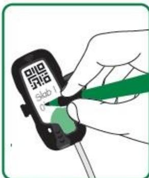
3 Assign the sensor a name in the mobile app and on its label
