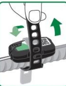
5 Pull strap tight over the installation hook and fold remaining strap over
