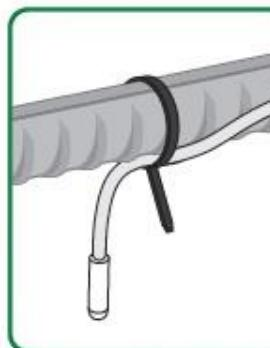
6 Secure the cable and temperature probe below the rebar
