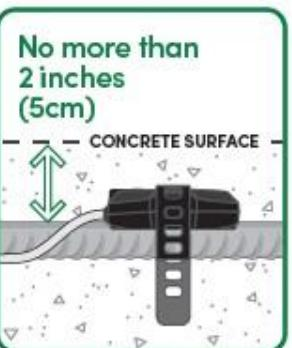
4 Install the transmitter on rebar no more than 2 inches (5cm) from concrete surface
