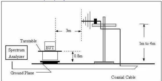
(C) Radiated Emission Test-Up Frequency Above 1GHz
