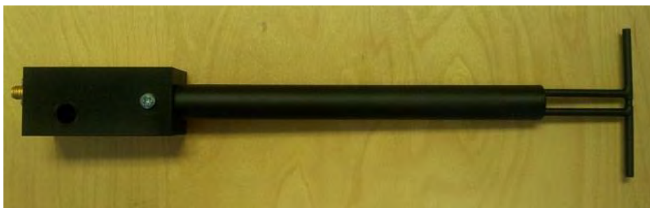
Figure 1 – MVG COMOSAR Validation Dipole
