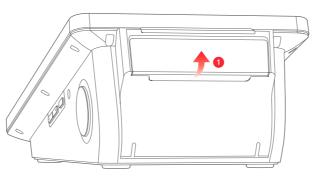
2 Insert the thermal paper and pull out part of it outside the paper exit of the printer, then close the paper compartment cover;
