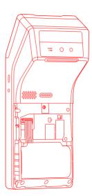
Open the battery cover: Insert the MicroSD Card, SIM Card as required:
