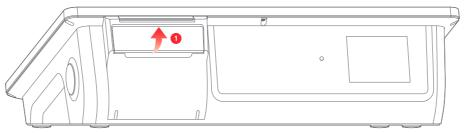
② Insert the thermal paper and pull out part of it outside the paper exit of the printer, then close the paper compartment cover;
