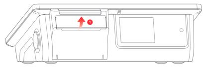
2 Insert the thermal paper and pull out part of it outside the paper exit of the printer, then close the paper compartment cover;
