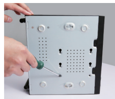
5. Secure the screws of the hard drive
