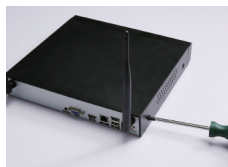
1. Remove the screws
