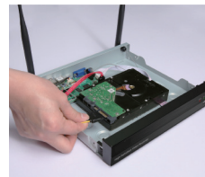
4. Connect the power wire
