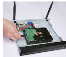
3. Connect the data wire
