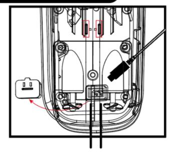
Unplug the charging cable cover and plug in the charging cable to charge. The lights on the hull will light up during charging, and the lights will go off when the battery is fully charged.
