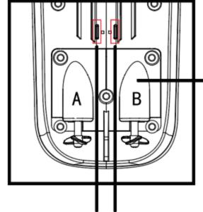
Replacing the propeller requires Corresponding to the blade The direction of A and B Corresponds to the hull
