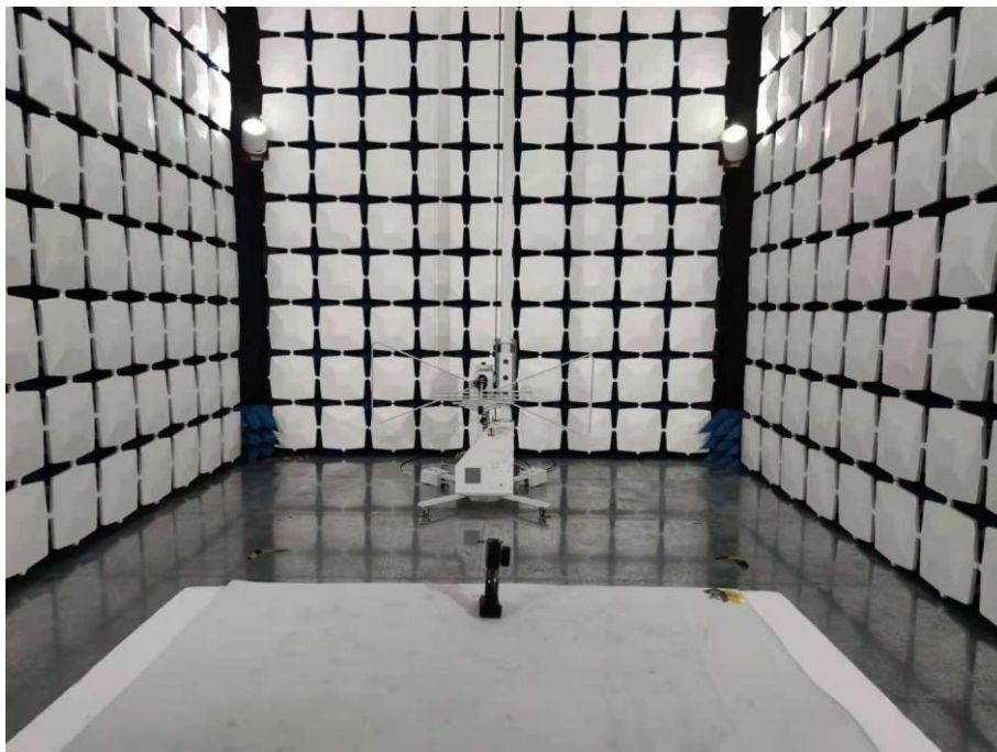
Below 1GHz for radiated emission test setup
