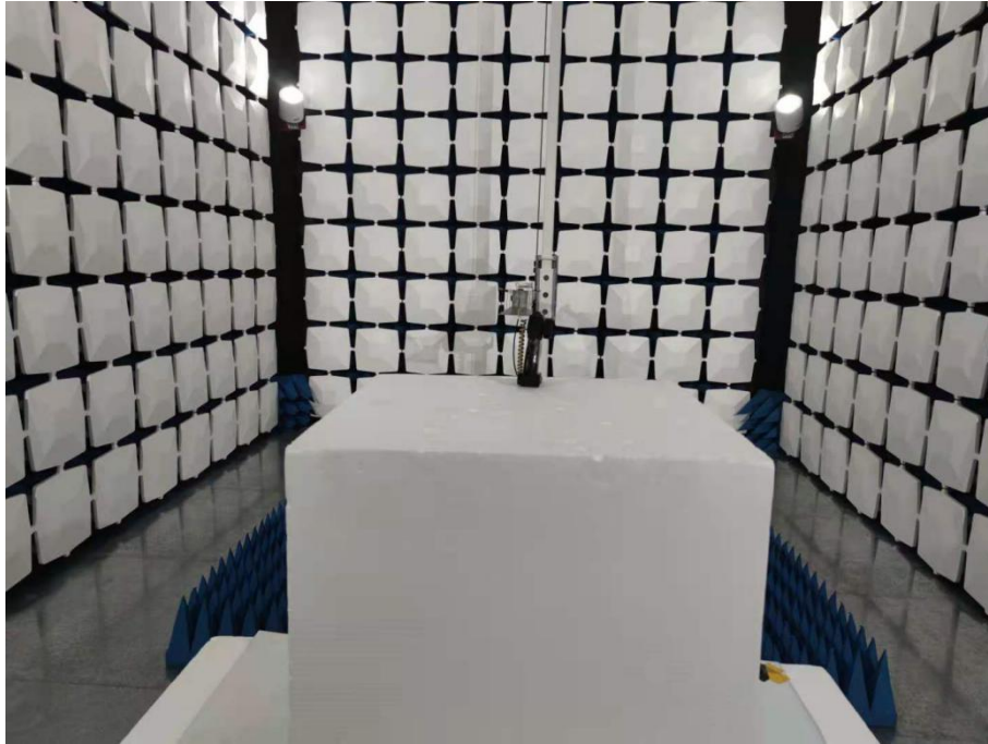
Above 1GHz for radiated emission test setup
