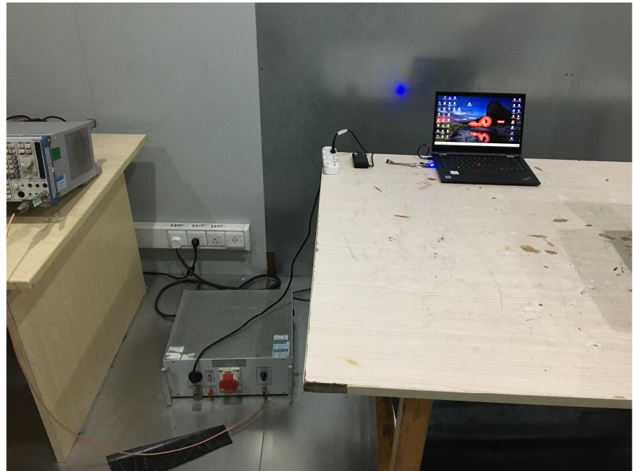
Conducted Emission Test Setup
