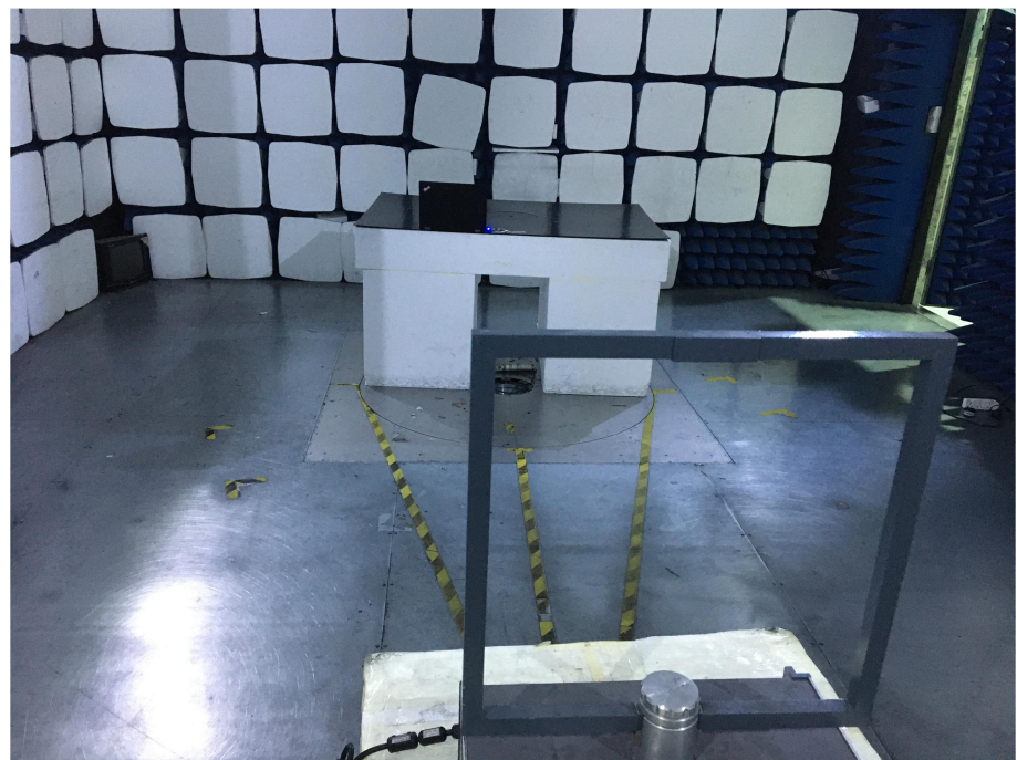
Radiation Emission Test Setup (Below 30MHz)
