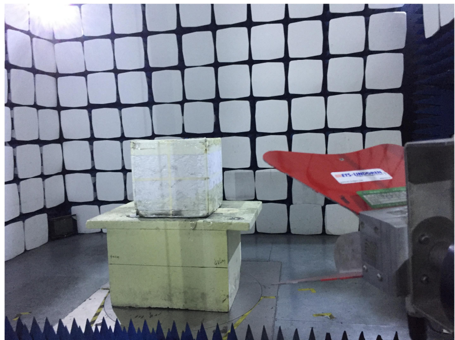
Radiation Emission Test Setup (1GHz to 18GHz)
