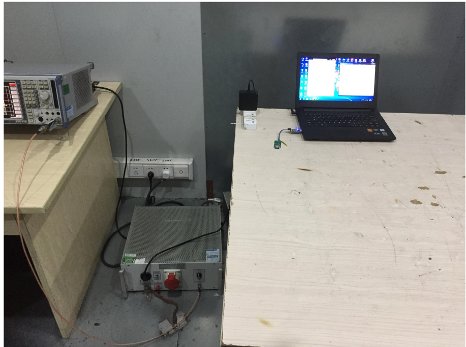
Conducted Emission Test Setup
