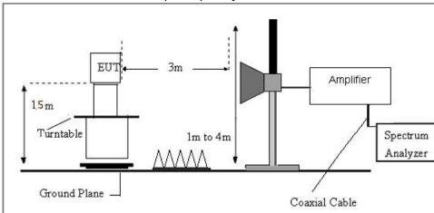
Radiated Emission Test-Up Frequency Above 1GHz
