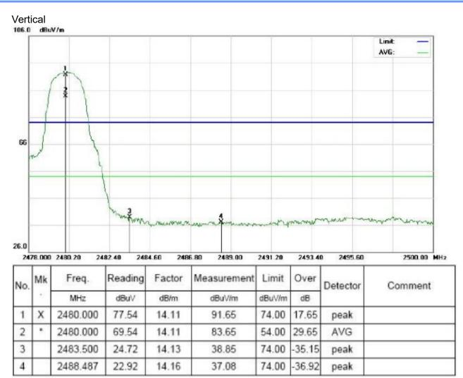
Note: Factor=Antenna Factor + Cable loss - Amplifier gain, Over=Measure-Limit.
