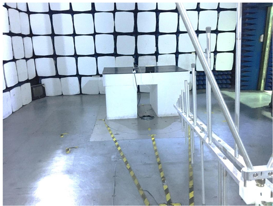
Radiation Emission Test Setup (30MHz to 1GHz)
