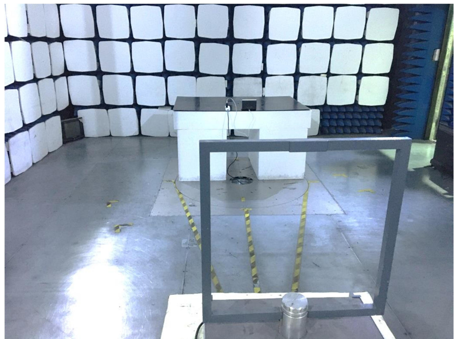
Radiation Emission Test Setup (Below 30MHz)
