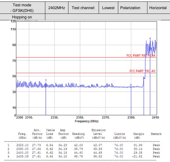
Remarks: 1. Emission Level= Antenna Factor + Cable Loss - Amp Factor + Reading. 2. The emission levels that are 20dB below the official limit are not reported.
