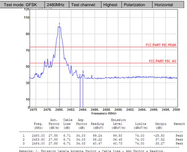
Remarks: 1. Emission Level= Antenna Factor + Cable Loss - Amp Factor + Reading. 2. The emission levels that are 20dB below the official
