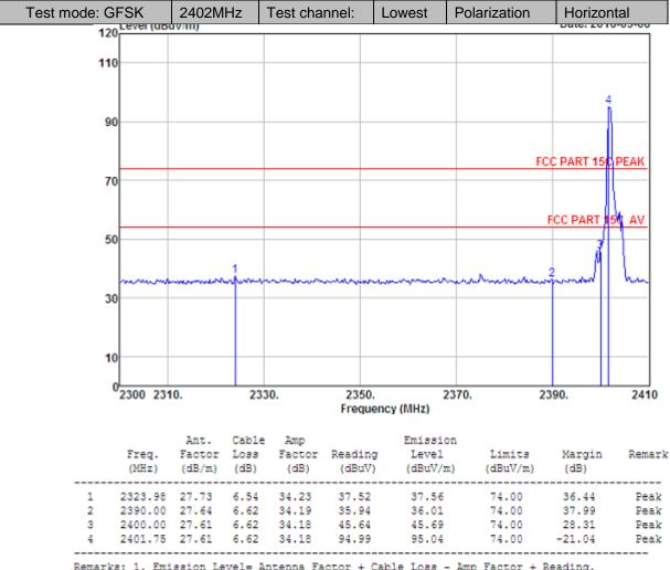
Remarks: 1. Emission Level= Antenna Factor + Cable Loss - Amp Factor + Reading. 2. The emission levels that are 20dB below the official
