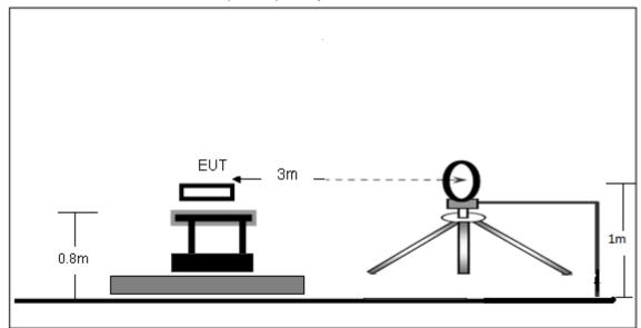
(B) Radiated Emission Test-Up Frequency 30MHz~1GHz
