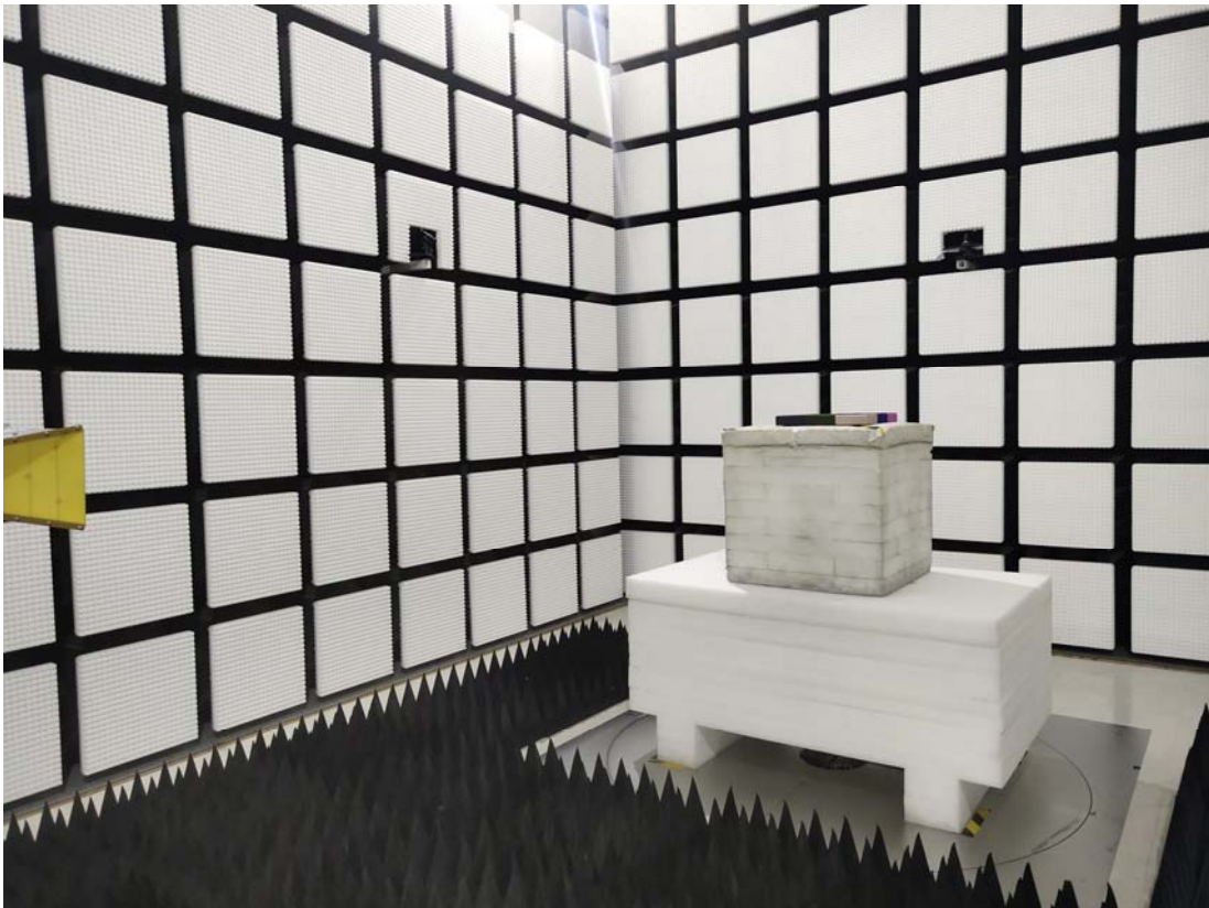
Radiated Emission Above 1GHz View
